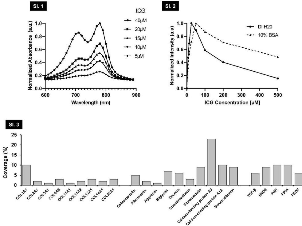
**Supplementary Figure 1:** Standard calibration curve for the absorbance of ICG using 40, 20, 15, 10, and 5  $\mu\text{M}$  concentrations in deionized water.
