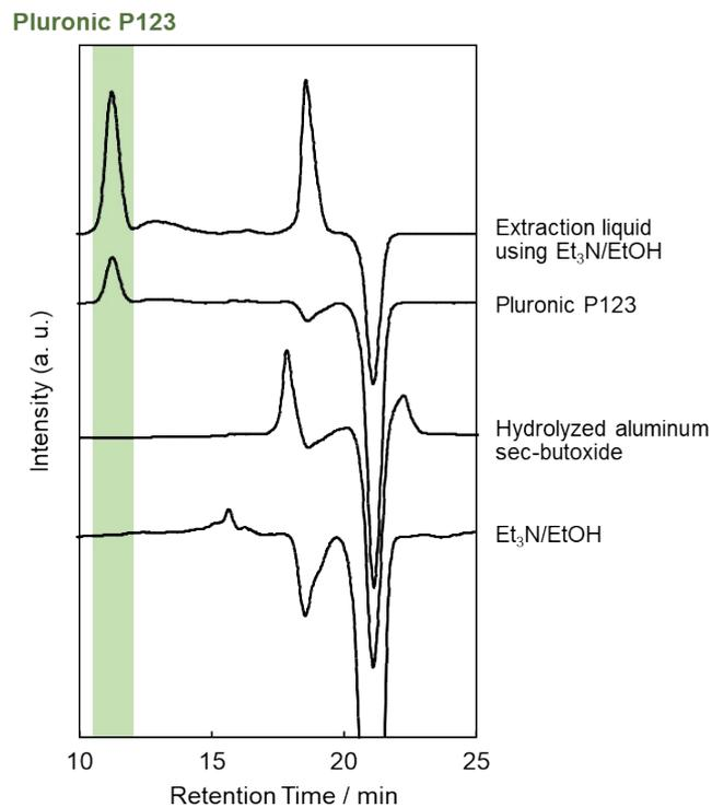
**Fig. S4** Size-exclusion chromatography (SEC) traces of resultant solutions after the neutralization-mediated extraction by using Et<sub>3</sub>N/EtOH.
