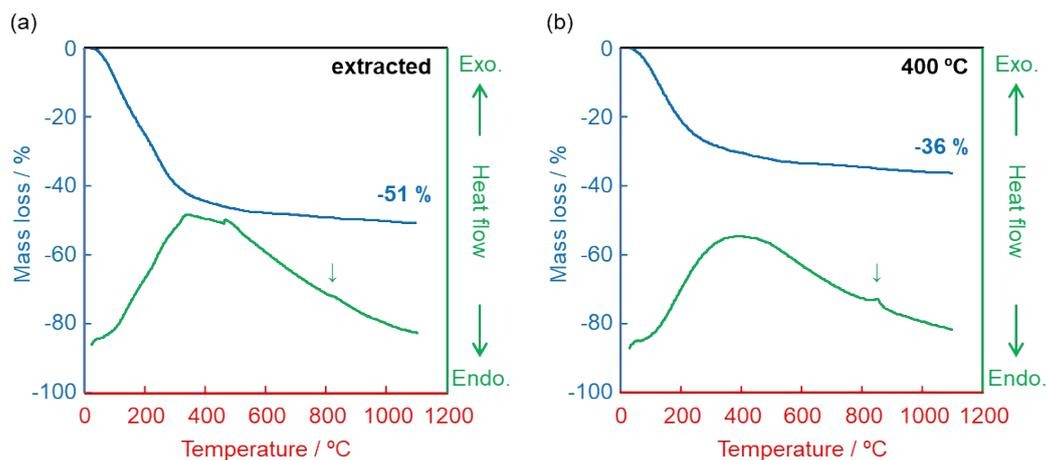
**Fig. S9** TG-DTA curves of mesoporous alumina (a) extracted by using  $\text{Et}_3\text{N}/\text{EtOH}$  and (b) calcined at  $400^\circ\text{C}$  without the extraction process. The green arrows ( $\downarrow$ ) show the exothermic peak due to crystallization to  $\gamma$ - $\text{Al}_2\text{O}_3$ .
