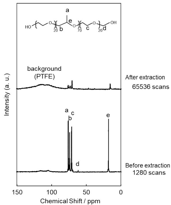
**Fig. S5** Solid-state  $^{13}\text{C}$  DD/MAS NMR spectra of successful mesoporous alumina before and after the neutralization-mediated extraction by using  $\text{Et}_3\text{N}/\text{EtOH}$ , with the assignment of signals to the molecular structure of Pluronic P123.
