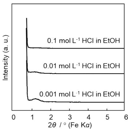
**Fig. S2** Low-angle XRD patterns after the treatment of a mesostructured alumina, prepared using Pluronic P123 under the HCl mediated acidic conditions, with ethanolic solution of gaseous HCl.
