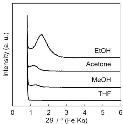
**Fig. S1** Low-angle XRD patterns after the treatment of a mesostructured alumina, prepared using Pluronic P123 under the HCl mediated acidic conditions, with some solvents.
