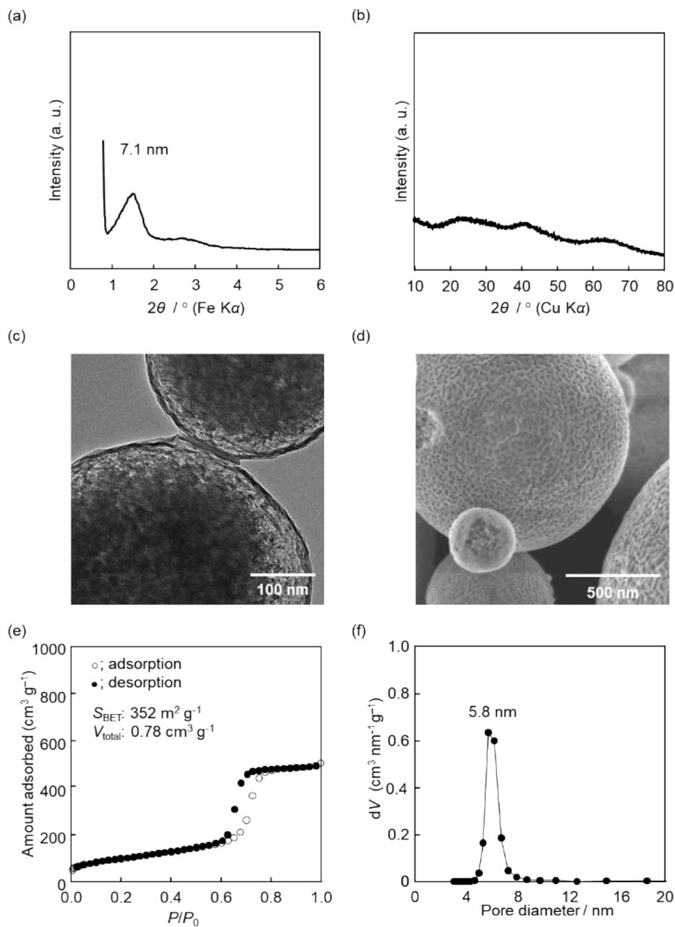
**Fig. S6** (a) Low- and (b) wide-angle XRD patterns, (c) TEM and (d) SEM images, and (e) N<sub>2</sub> adsorption-desorption isotherm with (f) corresponding pore size distribution curve of successful mesoporous alumina after the extraction by using Et<sub>3</sub>N/EtOH followed by calcination at 400 °C.
