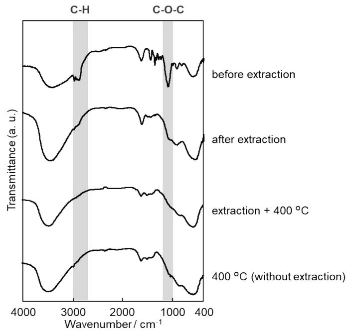
**Fig. S3** FT-IR spectra of a mesostructured alumina, prepared using Pluronic P123 under the HCl mediated acidic conditions and those after the neutralization-mediated extraction by using EtOH with triethylamine (Et<sub>3</sub>N), additional calcination at 400 °C and direct calcination at 400 °C without the extraction process.
