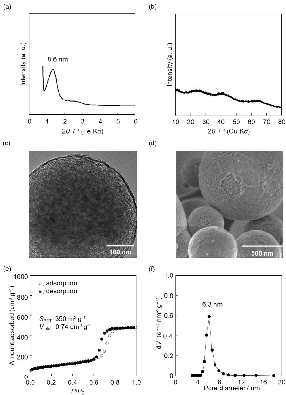
**Fig. S7** (a) Low- and (b) wide-angle XRD patterns, (c) TEM and (d) SEM images, and (e) N<sub>2</sub> adsorption-desorption isotherm with (f) corresponding pore size distribution curve of mesoporous alumina after the common calcination at 400 °C without the extraction process.
