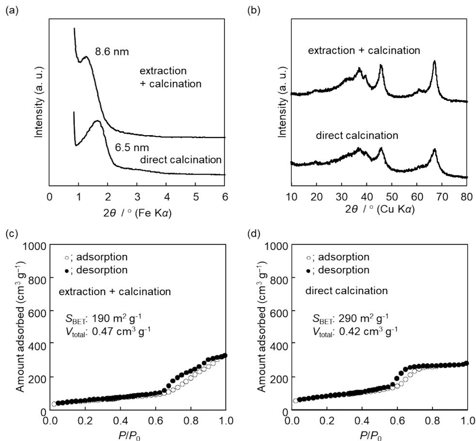
**Fig. S8** (a) Low- and (b) wide-angle XRD patterns and (c, d)  $\text{N}_2$  adsorption-desorption isotherm of mesoporous alumina calcined at  $850^\circ\text{C}$  for crystallization to  $\gamma$ - $\text{Al}_2\text{O}_3$ .
