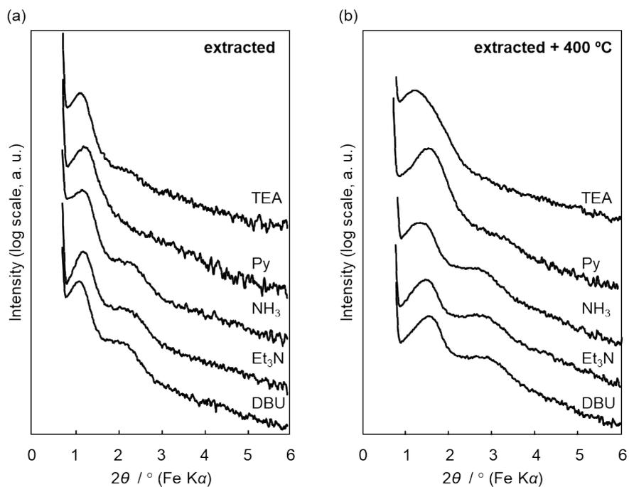
**Fig. S10** Low-angle XRD patterns of mesostructured alumina, prepared using Pluronic P123 under the HCl mediated acidic conditions (a) after the treatment by using EtOH in the presence of various amines followed by (b) calcination at 400 °C.
