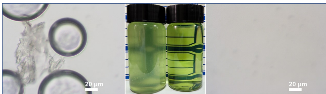
Fig. S15. Optical microscope photographs and digital photographs of the extract wastewater and its filtrate separated by the \text{Ti}_3\text{C}_2\text{Cl}_2\text{-(CuSA)}_5 membrane.
