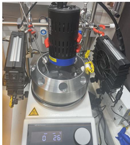
Reaction setup for synthesis of **4d** with Kessil lamp (160WE, PR 160 390 nm) in an aluminum holder.
