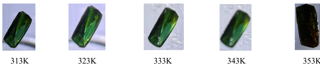
Figure S15. A crystal of complex 3 was placed on a diffractometer and photographed at different temperature (313 K to 353 K).
