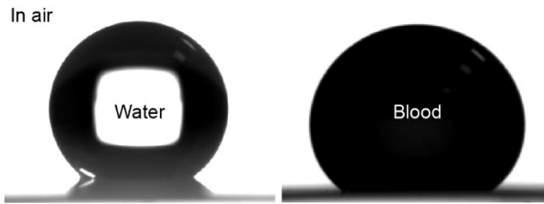
Fig. S3 Contact angles of water and blood droplets on the PP membrane in air.
