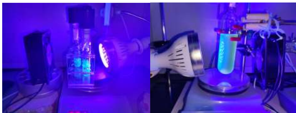
Figure S1. Reaction set up with a 30 W 390 nm LEDs (distance app. 2.0 cm from the bulb, left: model reaction; right: gram-scale reaction)
