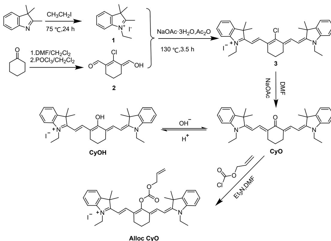
**Scheme S1.** Synthesis route of the fluorescent substrate (Alloc CyO).
