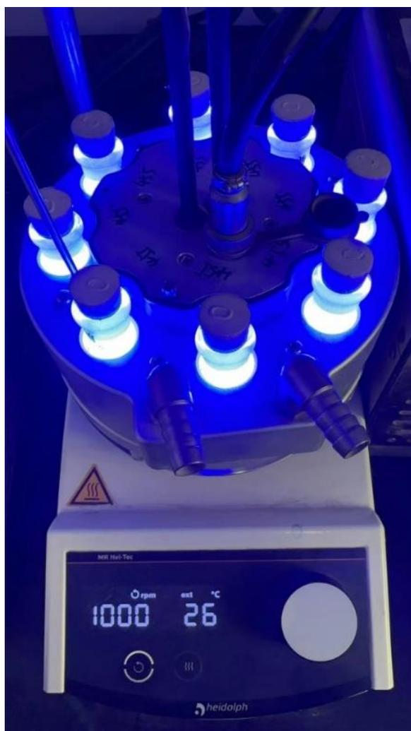
**Figure S1.** The Reaction Equipment and Light Source ( $\lambda_{\max} = 450 \text{ nm}$ ,  $\Delta\lambda = 25 \text{ nm}$ )
