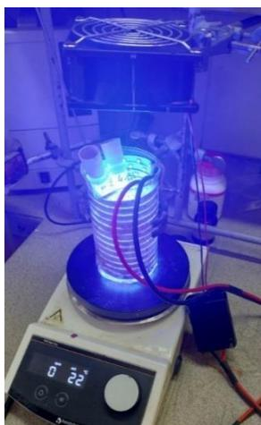
All photochemical reaction were performed in a beaker that contains blue LED tape (455 nm, 9 W) and are cooled with a fan.
