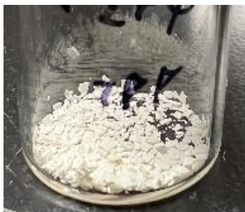
Fig. S8 A photograph of the recovered TPPW10 after the photocatalytic aerobic \alpha -oxygenation of 1a .
