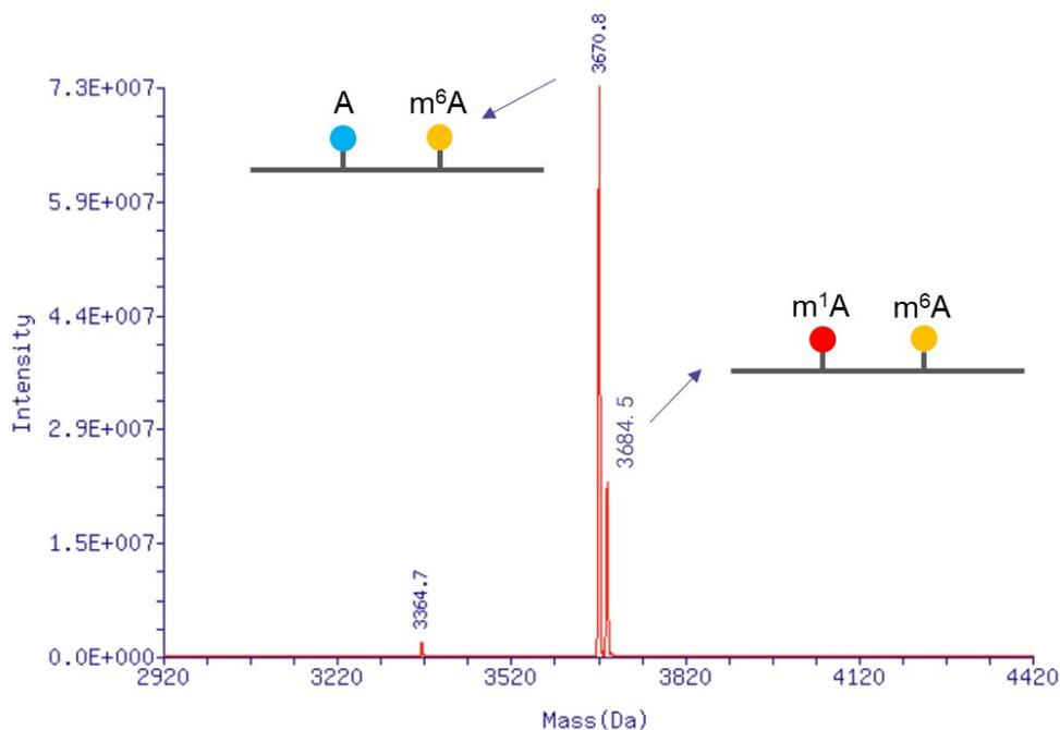
**Figure S2. ESI mass spectrometry for nucleotides after DMS reaction using RNA oligo containing both A and m<sup>6</sup>A (12 mer m<sup>6</sup>A-1). 3670.8 represents the mass before the reaction and 3684.5 represents the mass after the reaction.**
