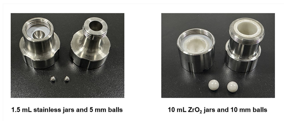
Figure S5. Stain-less and ZrO 2 jars and balls used in this study.
