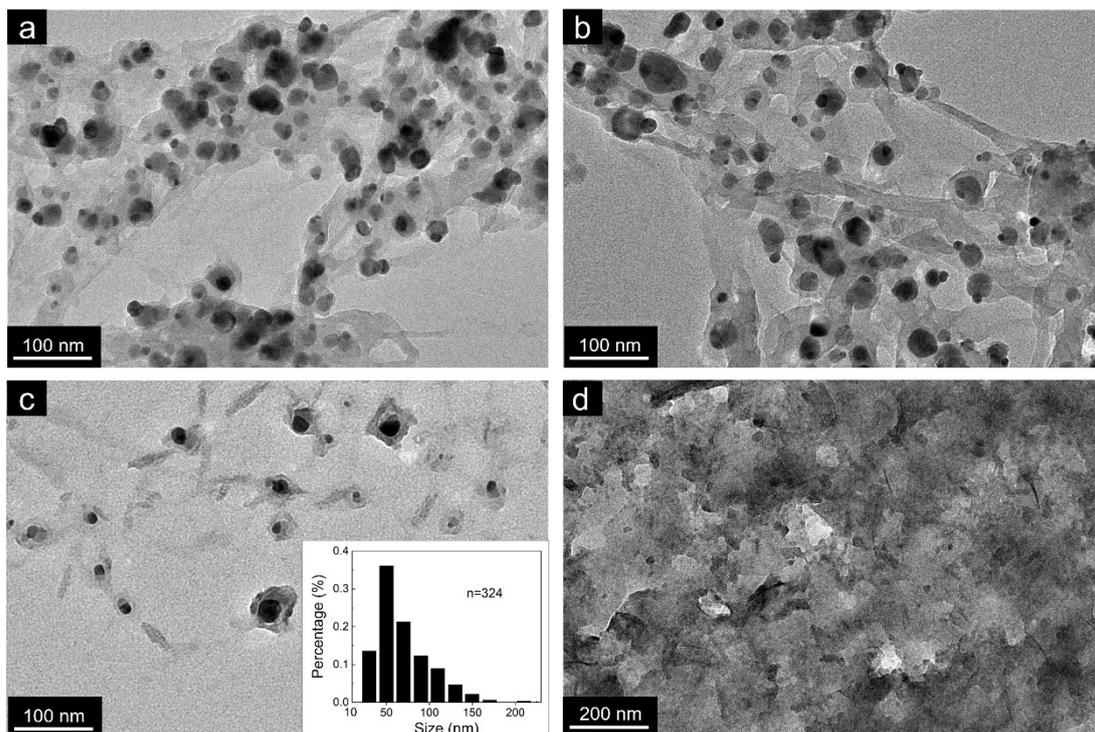
**Fig. S2.** TEM images of PANI/AgCl nanocomposites synthesized (a) in batch, (b) with soybean oil as ambient phase in the beaker, (c-d) in Janus droplet microreactors. The size distribution diagram of the nanoparticles produced in the Janus droplets is shown in the inset of (c).
