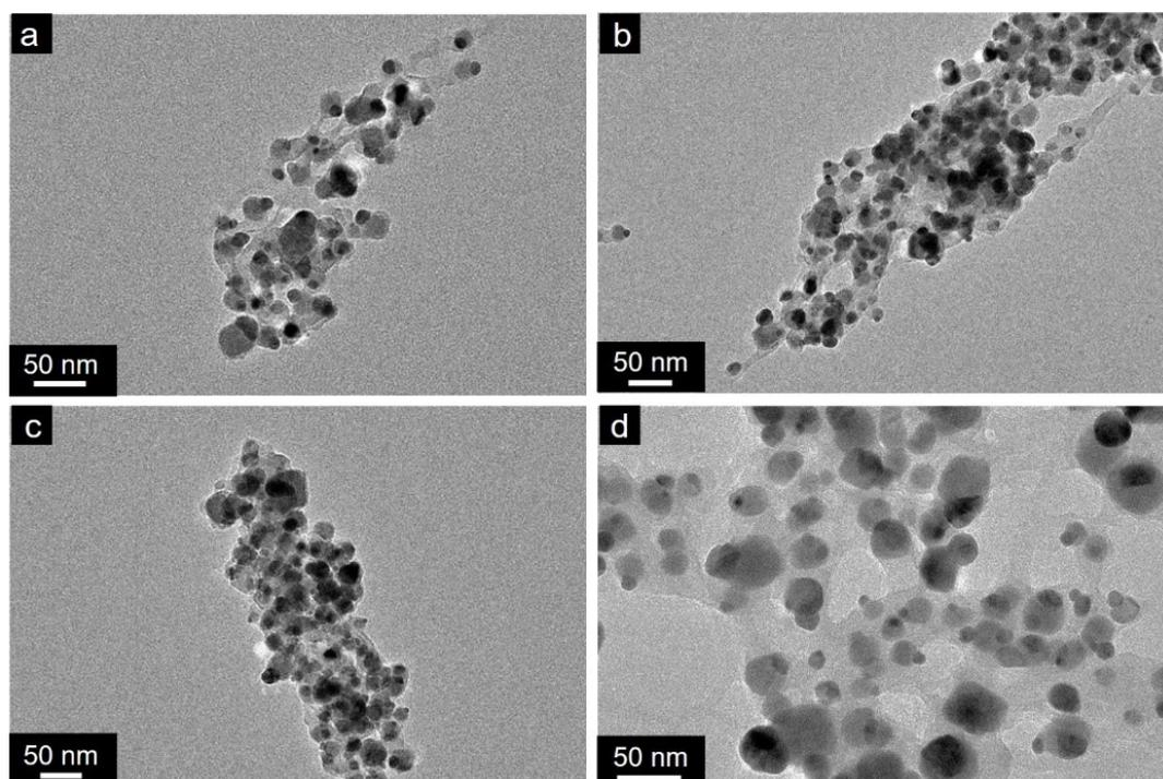
**Fig. S3.** TEM images of PANI/AgCl nanocomposites prepared in batch under different reaction times when the PVP concentration is 4%. (a) 2 h; (b) 3 h; (c) 5 h; (d) 24 h.
