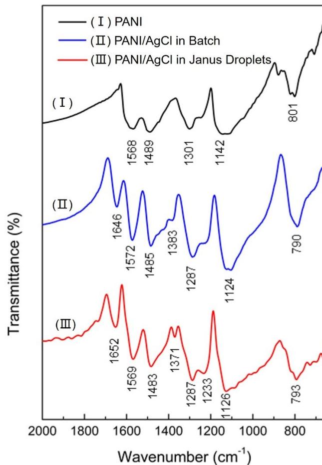
**Fig. S6.** FTIR spectrum of pure PANI (the black line I), AgCl/PANI nanocomposites prepared in batch (the blue line II) and AgCl/PANI nanocomposites synthesized via Janus droplet microreactors (the red line III).
