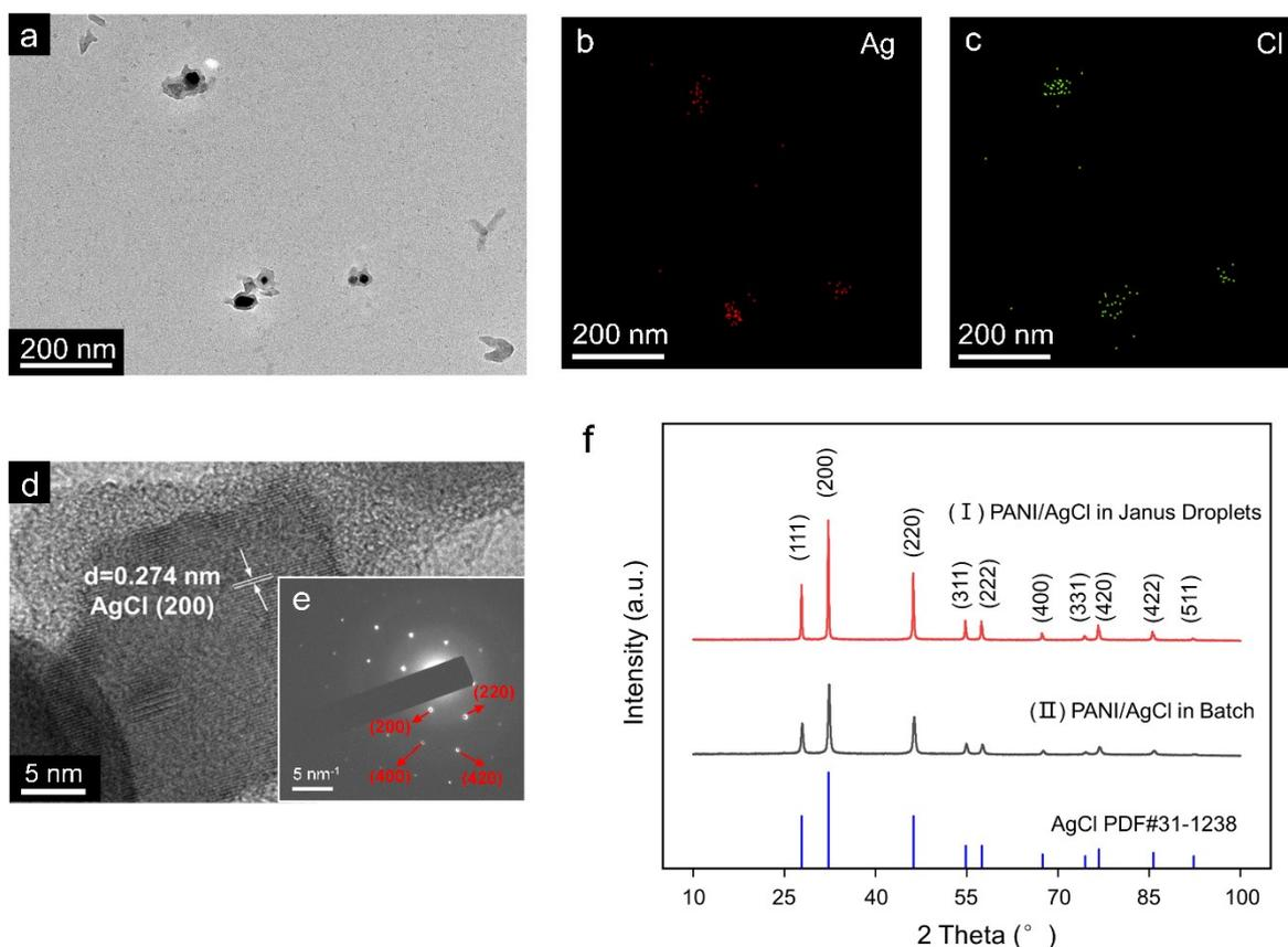
**Fig. S5.** (a) TEM image of PANI/AgCl nanoparticles synthesized in Janus droplet microreactors. (b-c) EDX element maps. (d) High-resolution TEM images of AgCl/PANI nanoparticles, whose lattices spacing value  $d$  of 0.274 nm was resolved, corresponding to AgCl (200) plane.<sup>33</sup> (e) SAED pattern of AgCl/PANI nanoparticles. (f) XRD patterns of PANI/AgCl nanocomposites prepared in batch (with soybean oil as the ambient phase in a breaker) and in Janus droplet microreactors.
