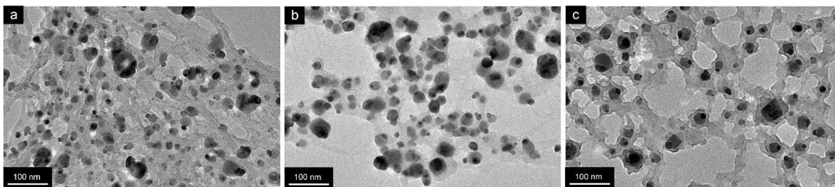
**Fig. S4.** TEM images of PANI/AgCl nanocomposites prepared in batch under different concentrations of PVP, (a) 0.5%; (b) 4%; (c) 8%.
