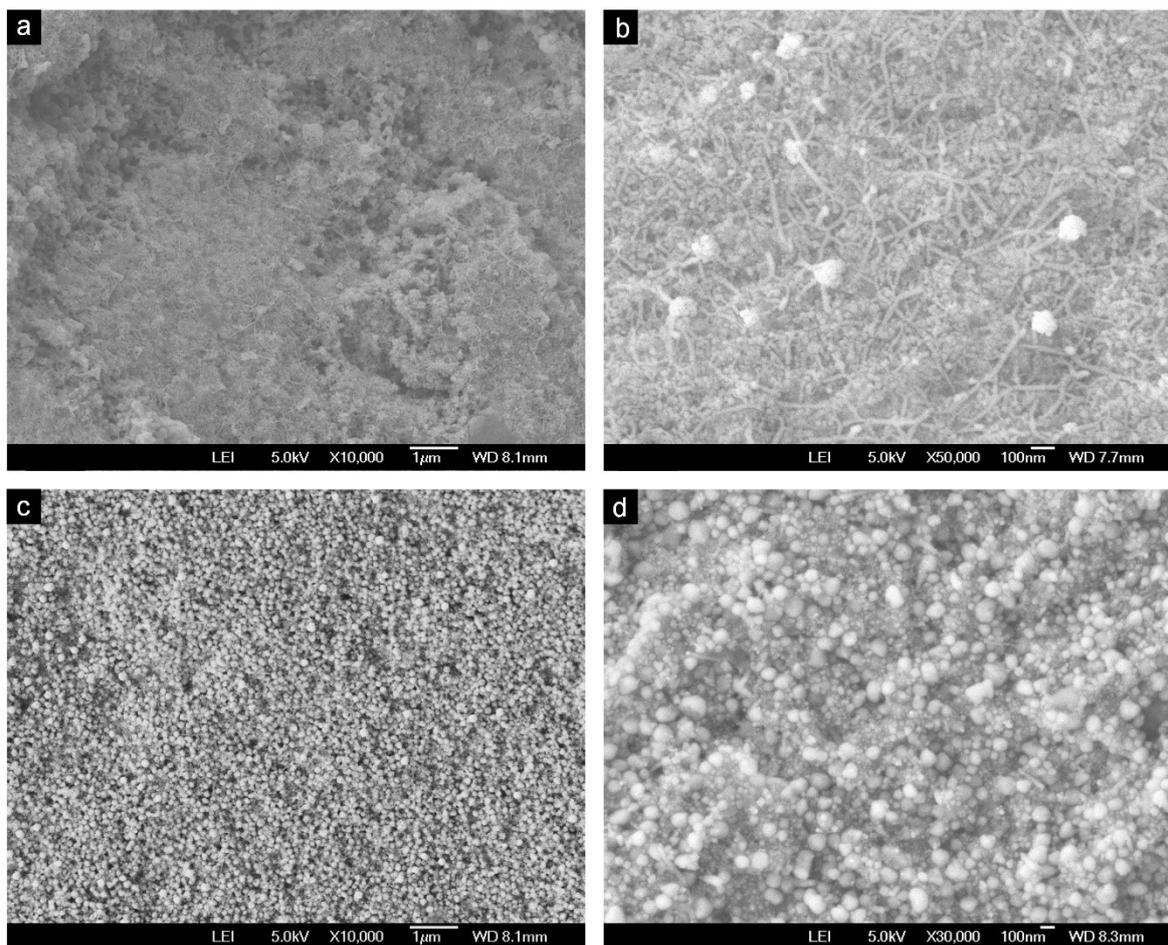
**Fig. S1.** SEM images of PANI/AgCl nanocomposites prepared (a-b) in batch (with soybean oil as the ambient phase in a breaker), (c-d) in Janus droplet microreactors.
