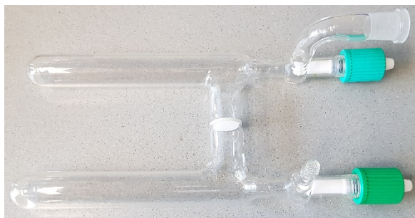
Figure S 1: Typical double-Schlenk tube which was used for all reactions.
