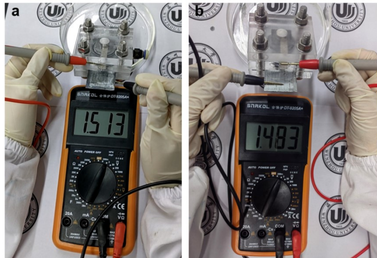
Fig. S28. The OCP for Ir-NC (a) and Pt/C (b) by measured with a multimeter.
