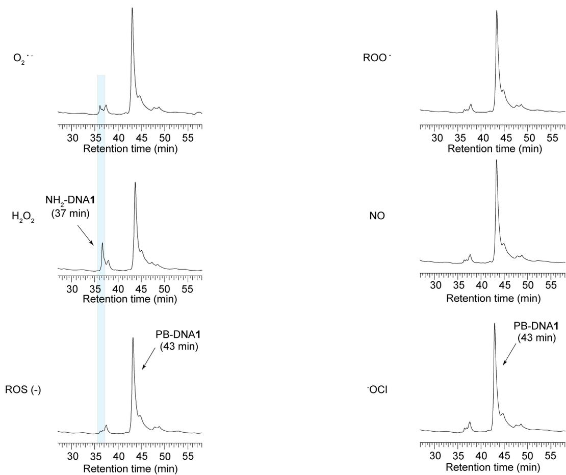
**Figure S3. Selectivity of PB-DNA for H<sub>2</sub>O<sub>2</sub>.** 5 μM PB-DNA1 reacted with 0 or 50 μM H<sub>2</sub>O<sub>2</sub>, potassium superoxide, NaOCl, NOC7 or AAPH in 250 mM phosphate buffer (pH 7.4) for 1 h at room temperature.
