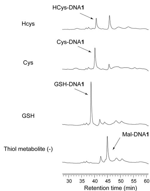
**Figure S8. Reaction monitoring of Mal-DNA1 and thiol metabolites** Reaction monitoring using HPLC; 5  $\mu$ M Mal-DNA1 reacted with 0 or 50  $\mu$ M GSH, Cys or HCys in 250 mM phosphate buffer (pH 7.4) for 1 h at room temperature.
