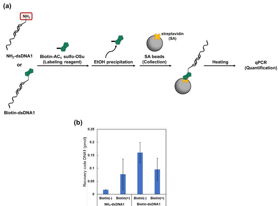
**Figure S4. Collection and detection of NH<sub>2</sub>-dsDNA1 by using biotin labelling.** (a) Schematic illustration of NH<sub>2</sub>-dsDNA1 or Biotin-dsDNA1 collection by using streptavidin coated magnetic beads. (b) Quantification of collected code DNA1 from NH<sub>2</sub>-dsDNA1 or Biotin-dsDNA1. Data = mean  $\pm$  SD (n=3).
