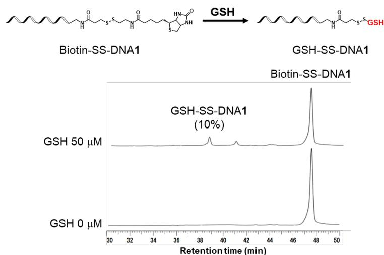
**Figure S7. Reaction monitoring of Biotin-SS-DNA1 and GSH** (ref 2). 5  $\mu$ M Biotin-SS-DNA1 reacted with 0 or 50  $\mu$ M GSH in PB (pH8.6, 250 mM) for 1 h at room temperature.
