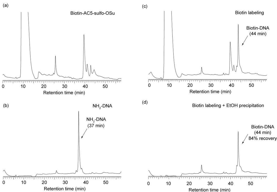
**Figure S5. Purification and recovery of biotin-DNA using the EtOH precipitation.** (a–c) Reaction monitoring using HPLC; 0 or 150 pmol  $\text{NH}_2\text{-DNA}_2$  was incubated with 0 or 1  $\mu\text{mol}$  biotin-AC5 sulfo-OSu in 200 mM carbonate-bicarbonate buffer (pH 8.7) for 1 h at room temperature. (d) After biotin labeling, the reaction solution was purified by using EtOH precipitation.
