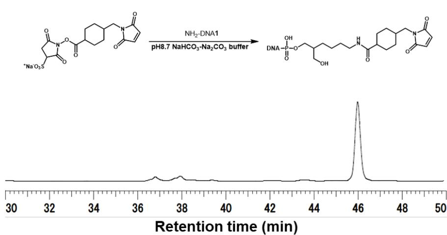
Figure S1. Synthesis of Mal-DNA1. HPLC chart of Mal-DNA1.
