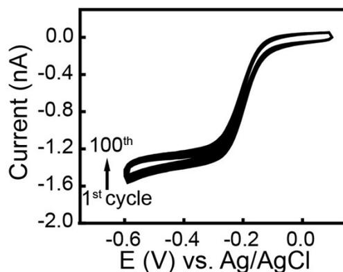
Fig. S3 Repetitive cyclic voltammograms (100 cycles) of 1 mM  $\text{Ru}(\text{NH}_3)_6^{3+}$ /1 M KCl of a SiC@Pt NWE.
