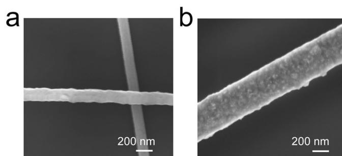
Fig. S2 SEM images of (a) SiC NWs and (b) SiC@Pt NW.
