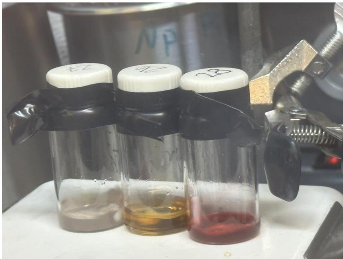
**Figure S17.** 1, 2, and 3 during synthesis in acetonitrile, pyridine, and toluene respectively.
