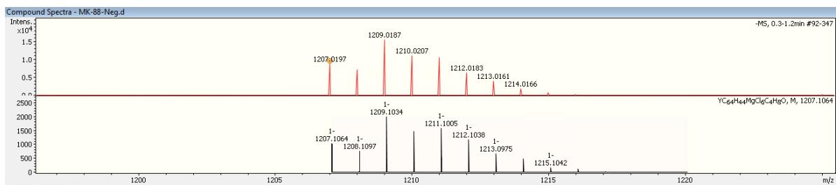
**Figure S5.** ESI-MS (-) of **3**.  $m/z$  expected for  $[M - Y(\text{THF})_5] = 1207.1064$ , found 1207.0197.
