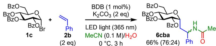
Glycosyl bromide **1c** (0.20 mmol, 132 mg), organic photocatalytic BDB (0.02 mmol, 8.3 mg), and potassium carbonate (0.40 mmol, 55.3 mg) were added to the dried Schrenk tube under argon. Dry MeCN (2.0 mL), styrene (**2b**) (0.4 mmol, 46 μL) and water (1.0 mmol, 18 μL) were added and stirred. Then the LED ramp was attached to the Schrenk tube using a Teflon joint, and freeze degassing were
