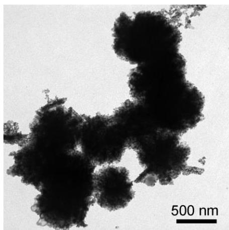
Fig. S1 TEM image of  $\text{Cu}_{0.20}\text{-Co}_9\text{S}_8\text{@CNFs}$  with the collapsed structures and CuS formation.
