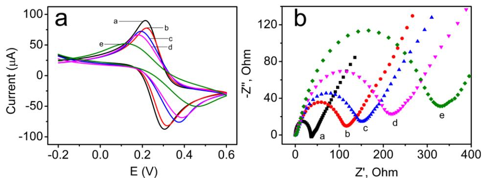
Fig. S13 (a) CV and (b) EIS characterizations of bare GCE (a),  $\text{Cu}_{0.15}\text{-Co}_9\text{S}_8@\text{CNFs}/\text{CNNS}/\text{a}$  (b), capture DNA/b (c), MCH/c (d), and CHA products/d (e) in 5 mM  $[\text{Fe}(\text{CN})_6]^{3-/4-}$  solution.
