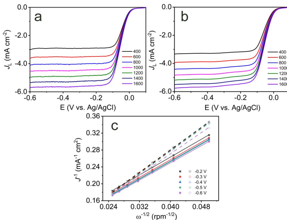
Fig. S2 LSV curves of (a)  $\text{Cu}_{0.15}\text{-Co}_9\text{S}_8@\text{CNFs}$  and (b) Pt/C measured in  $\text{O}_2$ -saturated 0.1 M KOH solution *via* RRDE at the rotating speeds of 400-1600 rpm, and (c) the corresponding Koutecky-Levich plots at the potentials of -0.20V~-0.60 V (vs. Ag/AgCl) (hollow:  $\text{Cu}_{0.15}\text{-Co}_9\text{S}_8@\text{CNFs}$ ; solid: Pt/C).
