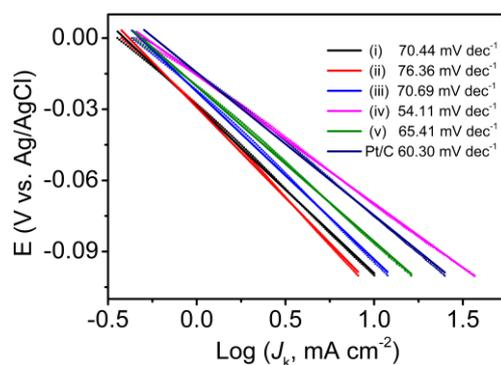
Fig. S3 Tafel plots (E vs.  $\text{Log}(J_k)$ ) of  $\text{Cu}_x\text{-Co}_9\text{S}_8@\text{CNFs}$  ( $x=0$  (i), 0.05 (ii), 0.10 (iii), 0.15 (iv), and 0.20 (v)) and Pt/C *via* LSV at 1600 rpm.
