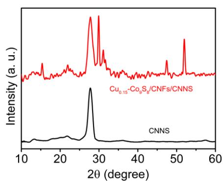
Fig. S7 XRD patterns of CNNS and  $\text{Cu}_{0.15}\text{-Co}_9\text{S}_8@\text{CNFs}/\text{CNNS}$ .
