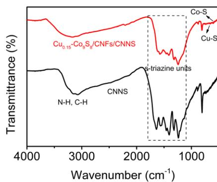
Fig. S8 FT-IR spectra of CNNS and  $\text{Cu}_{0.15}\text{-Co}_9\text{S}_8@\text{CNFs}/\text{CNNS}$ .
