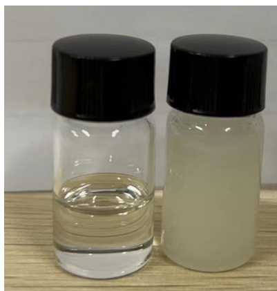
Figure S22 The image of MDEA-Im(1:1) before and after \text{SO}_2 absorption. (left: before capture; right: after capture)
