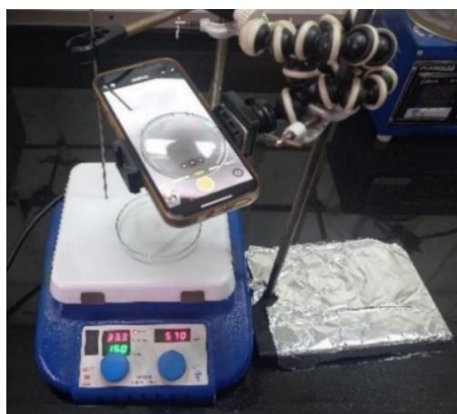
**Figure S6.** Hot stage setup to observe jumping at high temperature.
