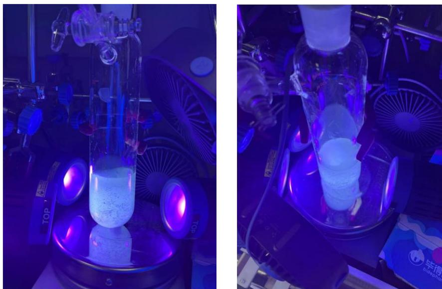
**Figure S2.** Photochemical set-up for large-scale reactions.
