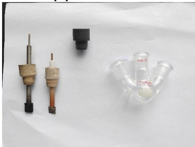
Figure S1 0.2 mmol scale electrolysis reaction set-ups: rubber plug, graphite plate (10 mm × 10 mm × 3 mm), platinum plate (10 mm × 10 mm × 0.1 mm) and 10 mL three-necked round bottom flask.
