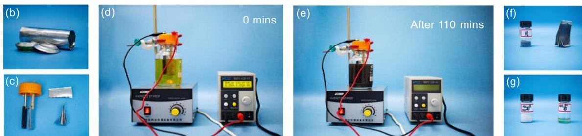
**Fig. S1** (a) Gram reaction of 1a (b) Discarded aluminium can (c) Anodes were prepared from waste aluminium cans (d) At the beginning of reaction (e) After the reaction (f) Recycled aluminium and anodes (g) Separated product
