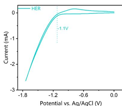
Fig. S2: CV spectra of HER at a scan rate of 50 mV s<sup>-1</sup>.
