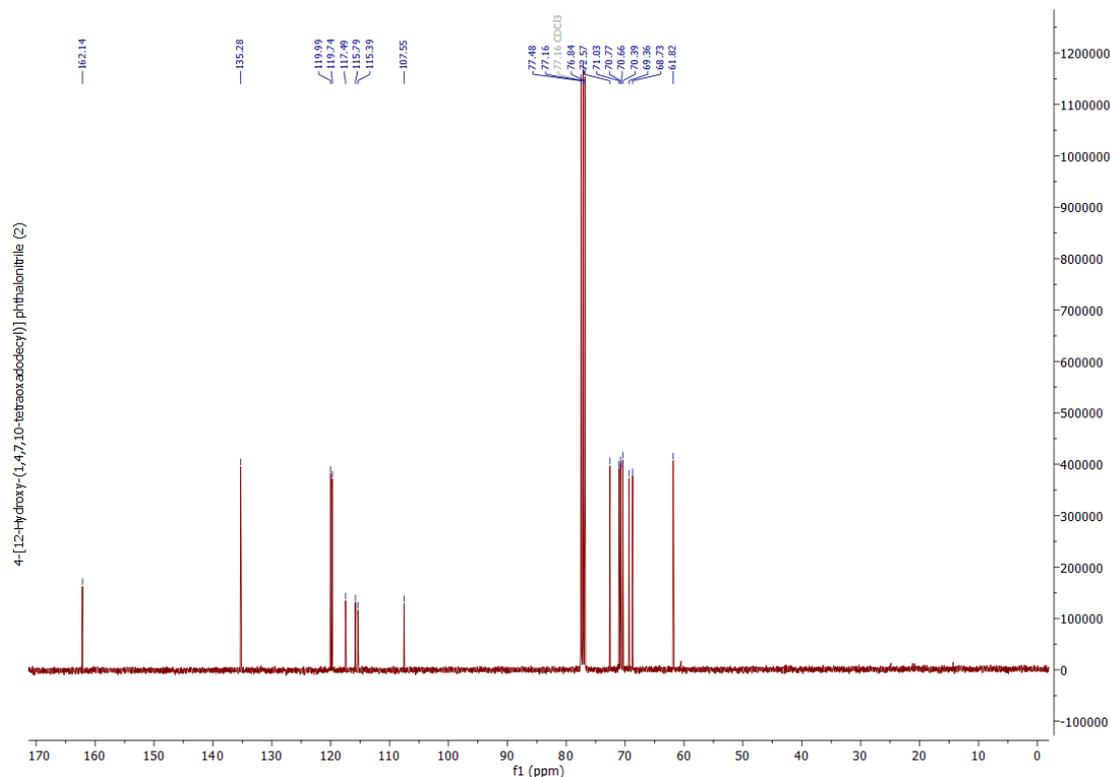
**Figure S17.**  $^{13}\text{C}\{^1\text{H}\}$ -NMR spectrum (101MHz,  $\text{CDCl}_3$ ) of 4-[12-Hydroxy-(1,4,7,10-tetraoxadodecyl)] phthalonitrile (**2**).
