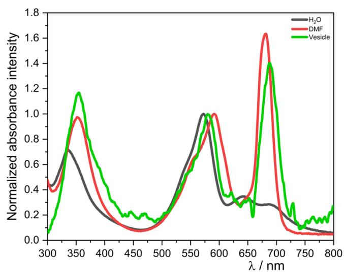
**Figure S5:** Normalized UV-vis absorption spectra of a suspension of αEGFR-mAb-P/P-aPSM-Cy3.5 nanocarriers (‘vesicle’) in H<sub>2</sub>O (green), referenced to the  $\lambda_{\text{max}}$  of Cy3.5. The spectra of aPSM-Cy3.5 in H<sub>2</sub>O and DMF are included for comparison (black dotted line and red dotted line, respectively) at 298 K.
