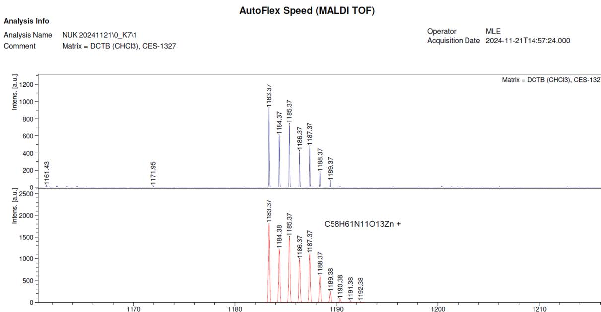
**Figure S22.** Mass spectrum (MALDI-ToF (DHB, CHCl<sub>3</sub>)) of [2(3),9(10),16(17)-tri-(2,2-dimethyl-1,3-dioxolan-4-yl)methoxy-23-(12-azido-1,4,7,10-tetraoxadodecyl)]phthalocyaninato Zn(II) (5).
