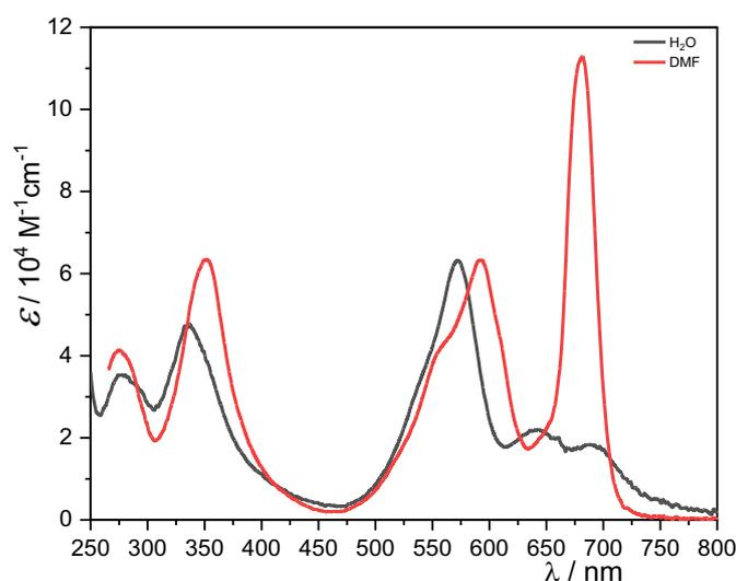
**Figure S1:** UV-vis absorption spectra (molar absorption coefficient as a function of wavelength) of aPSM-Cy3.5 in H<sub>2</sub>O (black) and DMF (red). Validity range:  $c = 10^{-6} - 10^{-4}$  M at 298 K.
