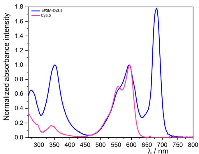
**Figure S3:** Normalized UV-vis absorption spectra of **aPSM-Cy3.5** (blue) and **Cy3.5** (pink) in  $\text{DMF}$  at 298 K, referenced to the  $\lambda_{\text{max}}$  of **Cy3.5**.
