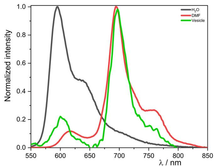
**Figure S6:** Normalized emission spectra ( $\lambda_{\text{ex}} = 500 \text{ nm}$ ) of a suspension of  $\alpha\text{EGFR-mAb-P/P-aPSM-Cy3.5}$  nanocarriers ("vesicle") in  $\text{H}_2\text{O}$  (green). The spectra of **aPSM-Cy3.5** in  $\text{H}_2\text{O}$  and DMF are included for comparison (black dotted line and red dotted line, respectively) at 298 K.
