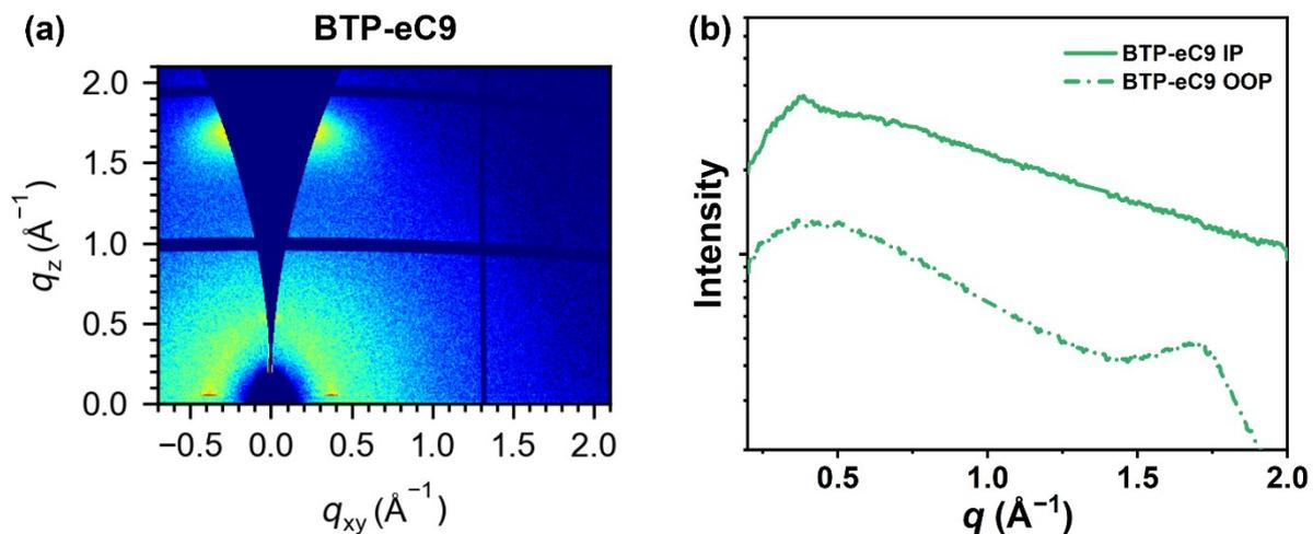
**Fig. S8** (a) 2D GIWAXS pattern and (b) the corresponding line cut profiles of neat BTP-eC9 film.
