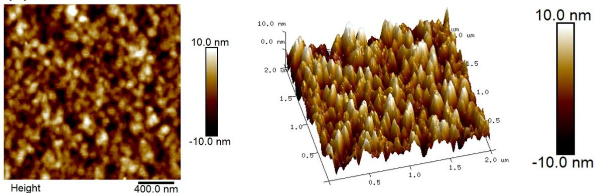
**Fig. S7** AFM height images of PPAF:BTP-eC9 and PPAT:BTP-eC9 films.
