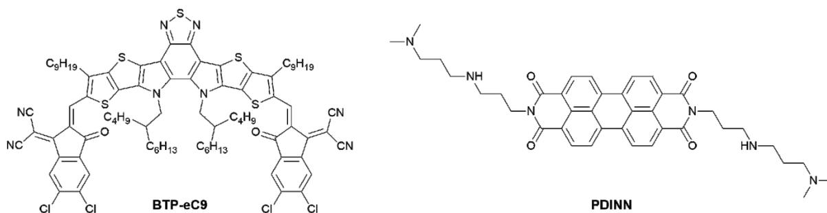
**Fig. S5** The molecular structures of BTP-eC9 and PDINN.
