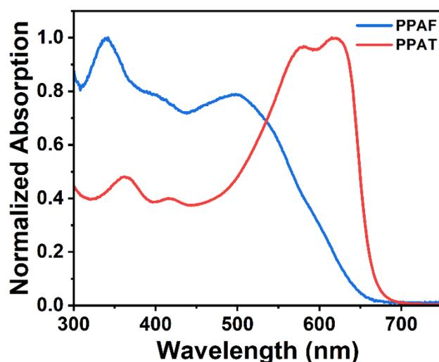
**Fig. S3** The normalized absorption spectra of PPAF and PPAT chloroform solutions.
