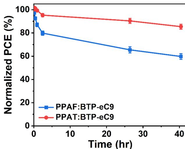
**Fig. S6** Normalized PCEs of the devices under continuous 1 sun illumination of an array of white LED. Average PCEs and error bars are calculated from eight devices.
