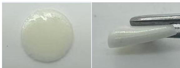
Figure S4. Photographs of the CSE electrolyte under original and folding states.
