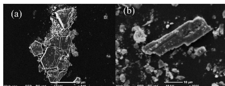
Fig. S9 Scanning electron microscopic images for 1 (a) before adsorption experiments and (b) after adsorption experiments.
