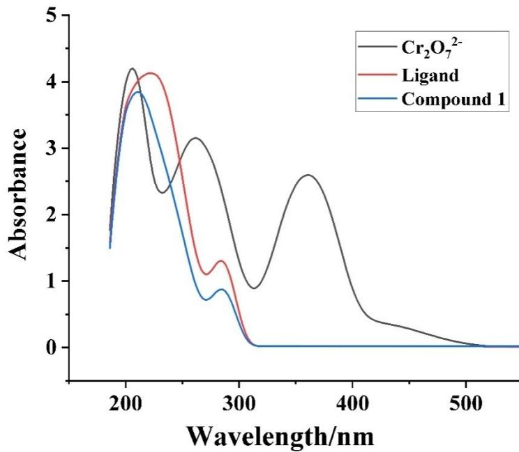
Fig. S5 The spectral overlap between the emission spectra of **1** and bip ligand with the Uv-Vis spectrum of dichromate anion.
