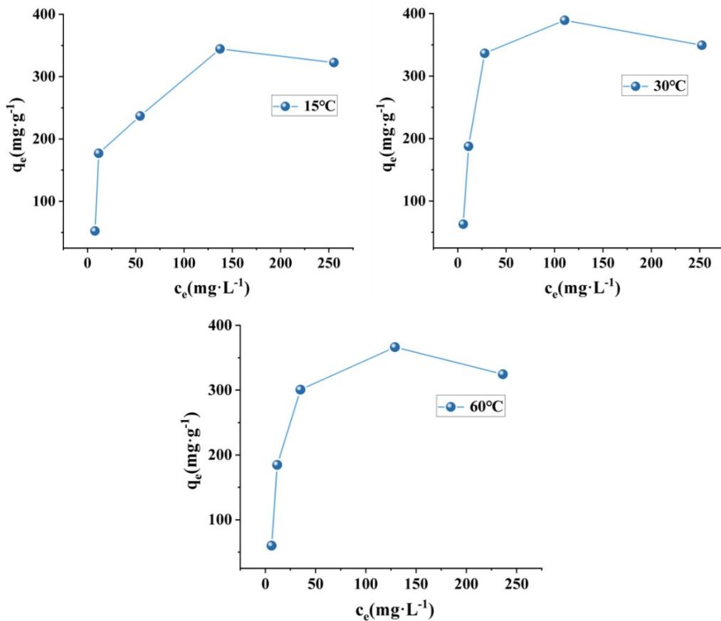
Fig. S6 Adsorption isotherms for dichromate adsorption over **1** at 288, 303 and 333 K
