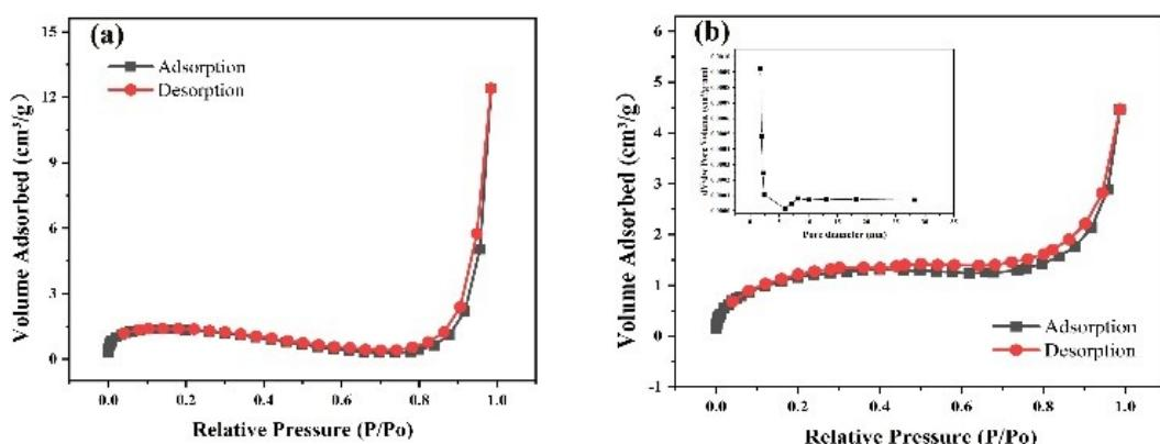
Fig. S8 The BET surface area analyses (a) before and (b) after adoption Cr<sub>2</sub>O<sub>7</sub><sup>2-</sup> anion.
