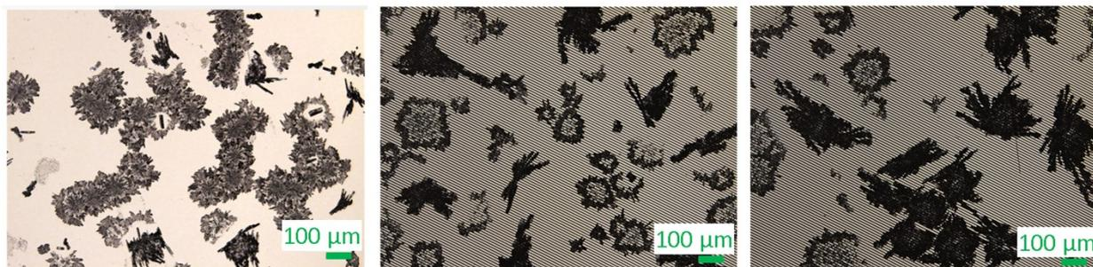
**Figure S8.** Laser microscope images of the 1  $\mu\text{m}$  samples after annealing at 120  $^{\circ}\text{C}$  (30 min) on sapphire substrate (a) over the IDE (b). Fig (c) shows the laser microscope image for the 1  $\mu\text{m}$  sample annealed at 150  $^{\circ}\text{C}$  (15 min) on IDE.
