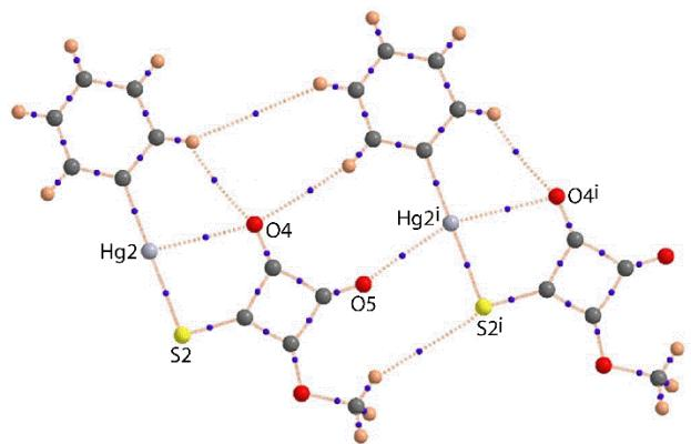
**ESI Figure S14.** QTAIM analysis (BCPs are represented as blue spheres and bond paths as dotted orange lines) highlighting the Hg···O spodium bonding involving the second independent molecule of **PhHgL<sup>Me</sup>**.
