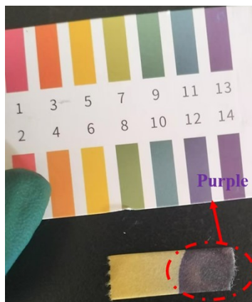
Figure S1 The pH test paper for mixed solution of \text{Cs}_2\text{CO}_3 , \text{HBr} and \text{PbBr}_2 with methylamine vapor.
