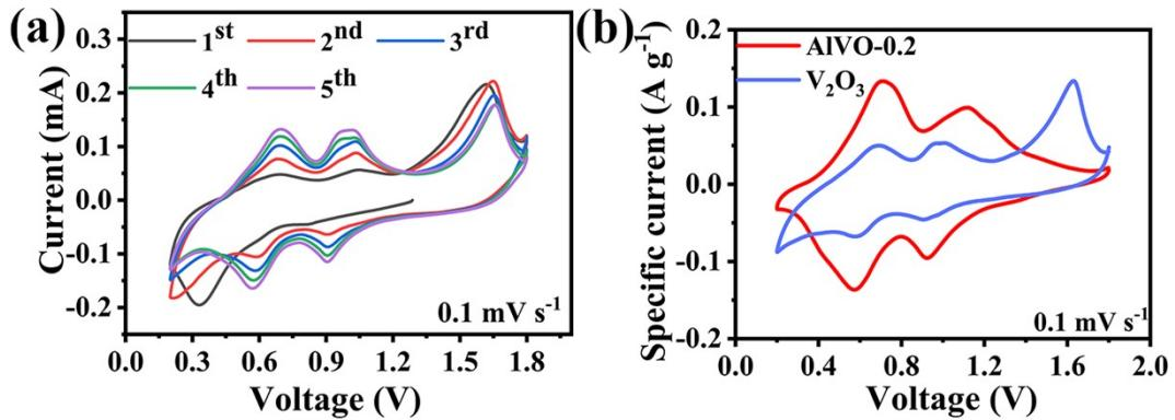
S5. (a) CV curves of  $\text{V}_2\text{O}_3$  at  $0.1 \text{ mV s}^{-1}$ , (b) Comparison of CV curves of  $\text{V}_2\text{O}_3$  and AlVO-0.2 at  $0.1 \text{ mV s}^{-1}$ .
