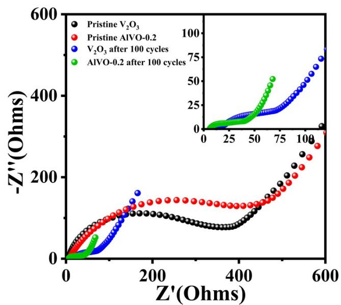
S9. EIS plots of  $\text{V}_2\text{O}_3$  and AlVO-0.2 cathode before and after cycle.
