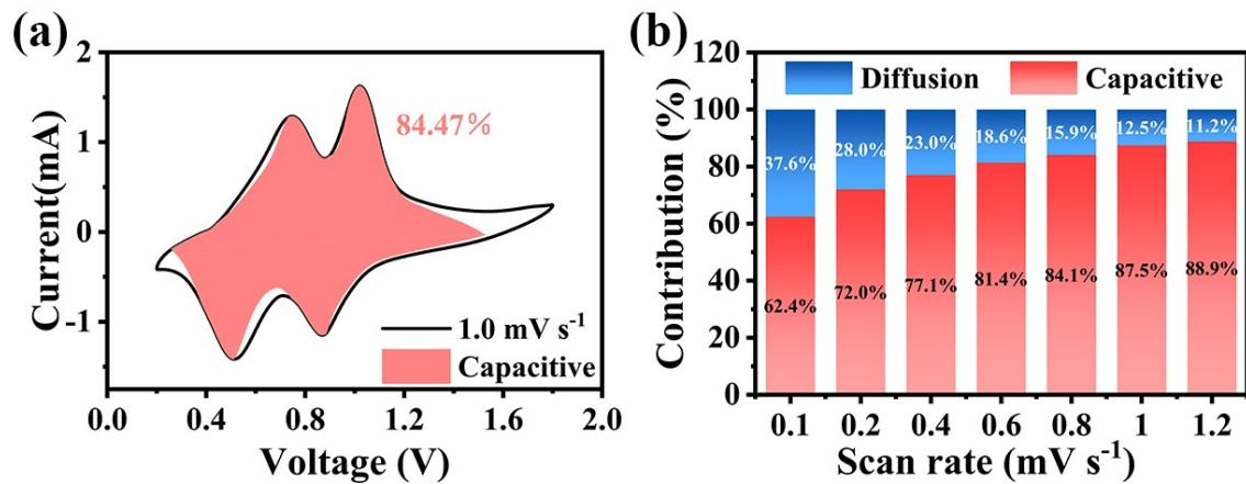
S6. (a) Pseudocapacitance contribution ratio at the current density of  $1.0 \text{ mV s}^{-1}$ . (b) Capacitance contribution at different scan rates of  $\text{V}_2\text{O}_3$  cathode.
