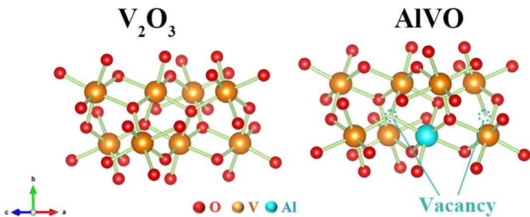
S3. Crystal structure schematic of pure V<sub>2</sub>O<sub>3</sub> and AlVO.
