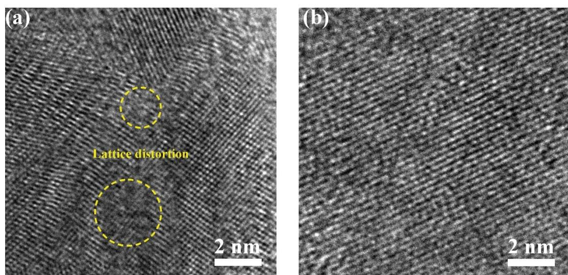
S2. HRTEM image of AlVO-0.2 and undoped- $\text{V}_2\text{O}_3$ .
