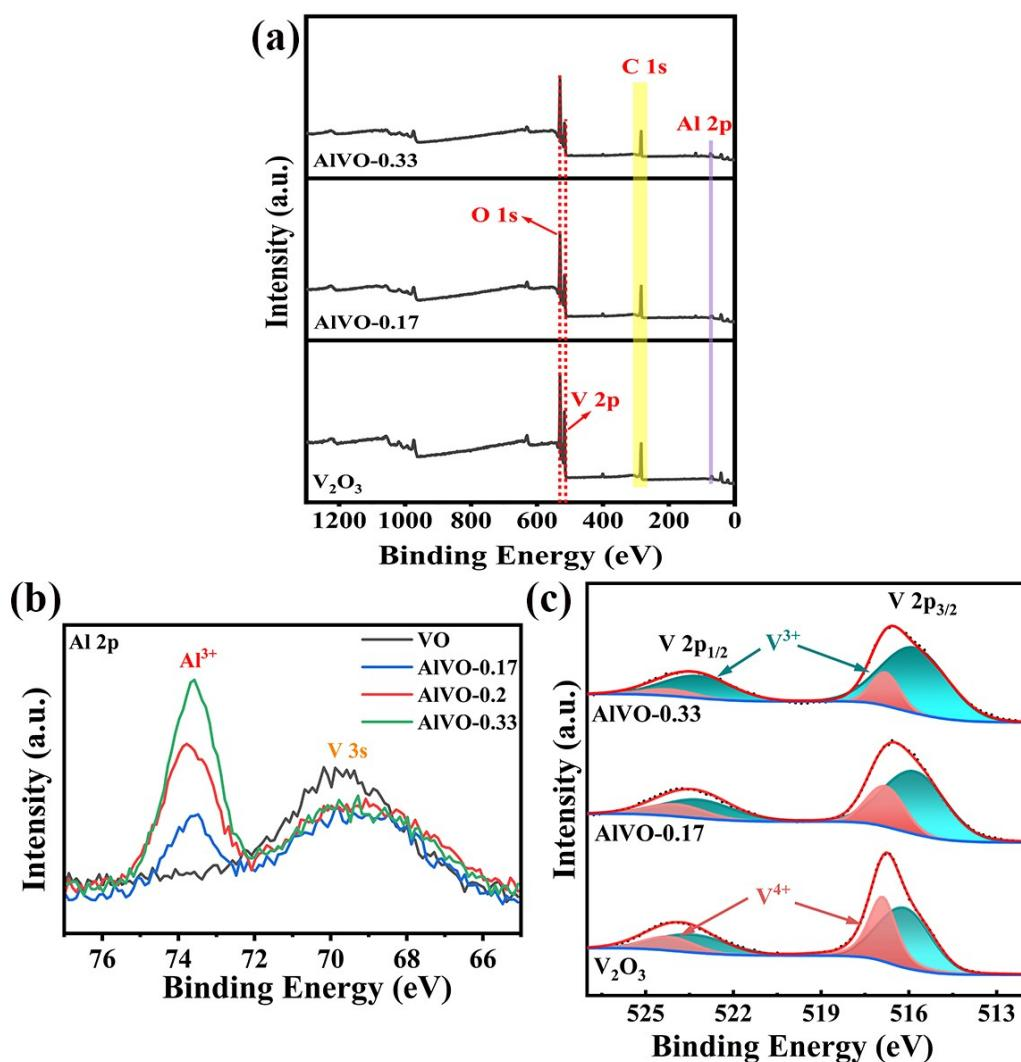
S4. (a) XPS full survey spectra, (b) Al 2p and (c) V 2p of V<sub>2</sub>O<sub>3</sub>, AlVO-0.17 and AlVO-0.33 samples.
