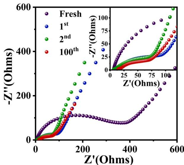
S7. EIS plots of  $\text{V}_2\text{O}_3$  cathode in different stages.
