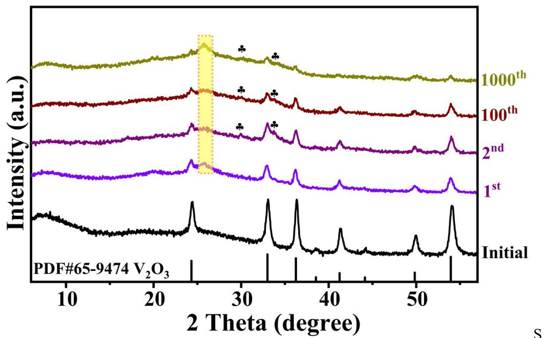
8. Ex situ XRD analysis of the  $\text{V}_2\text{O}_3$  cathode at various states
