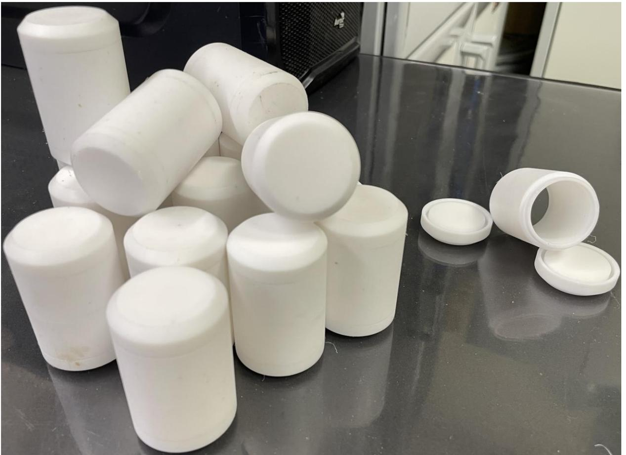
**Photograph S5.** Teflon ampoules with an internal volume of 22 cm<sup>3</sup>.
