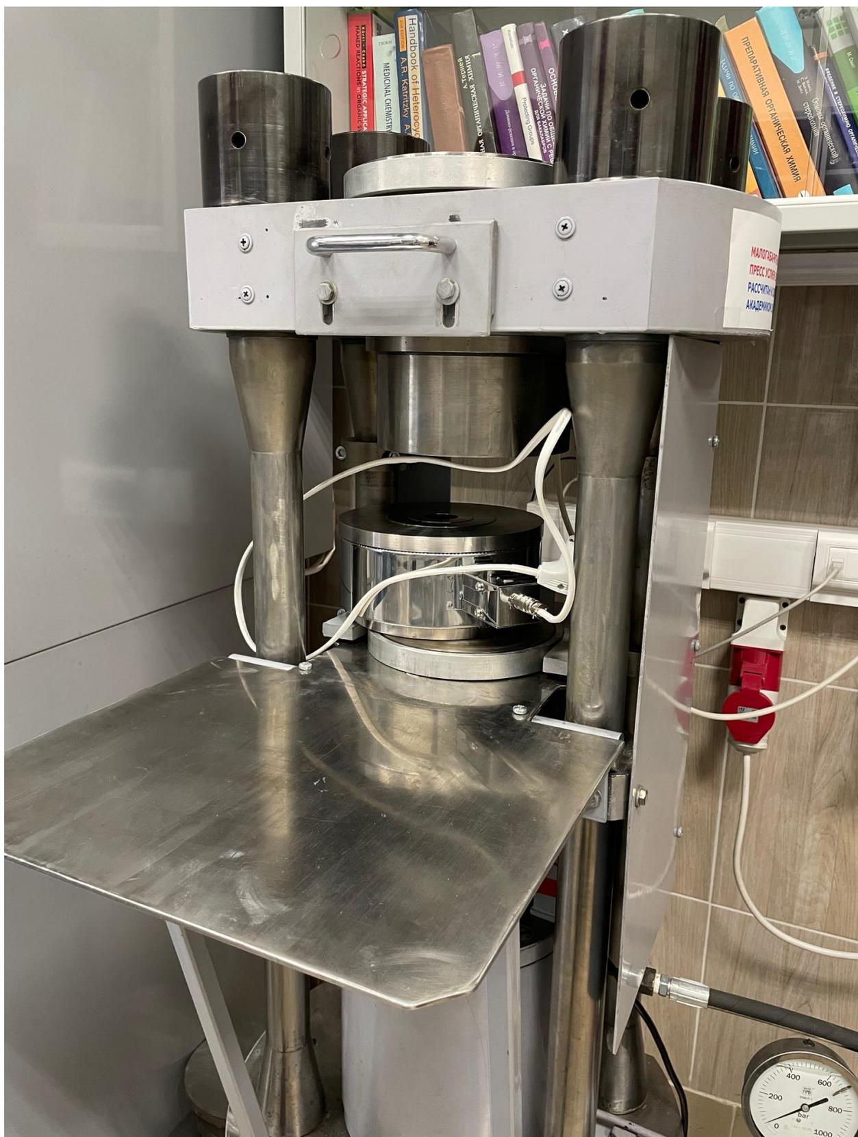
**Photograph S3.** Cell with a piston-cylinder chamber and a heating element
