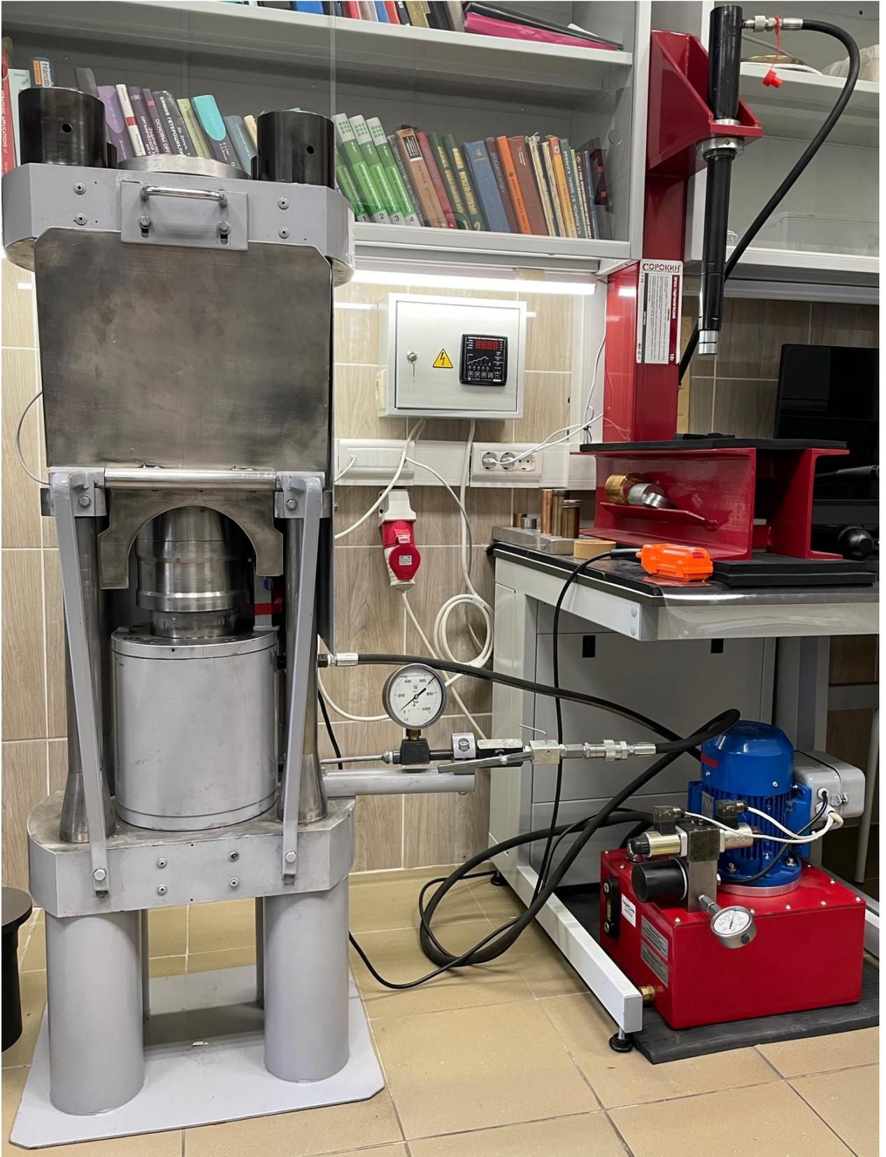
**Photograph S2.** Hyperbaric apparatus with a closed steel protective cell door of a piston-cylinder chamber
