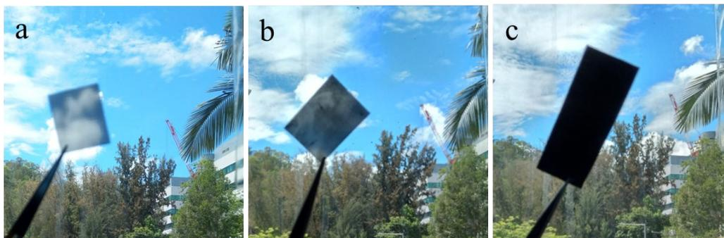
**Figure S3.** Optical photographs of SS/VS<sub>2</sub> prepared with three different mass loadings (a) 1 mmol to 7.5 mmol (b) 2 mmol to 15 mmol (c) 3 mmol to 22.5 mmol
