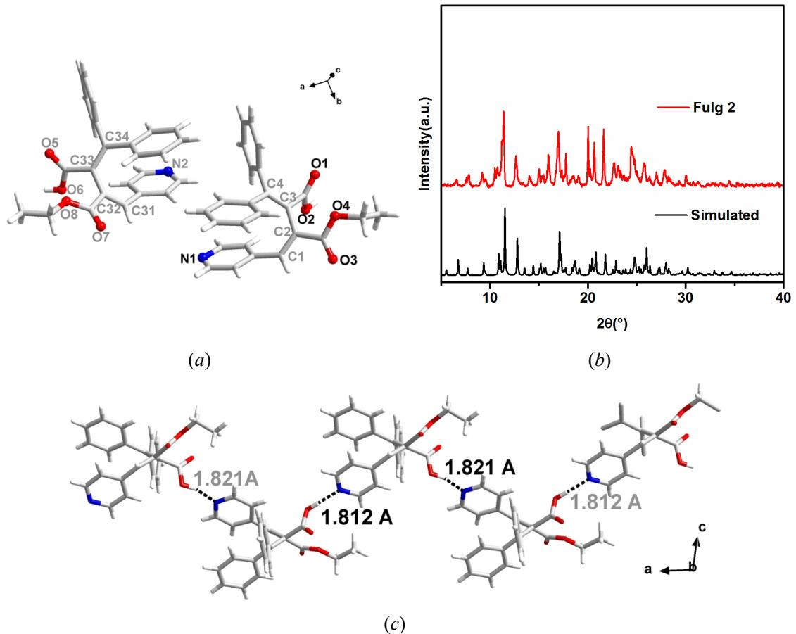
**Figure S19.** (a) Molecular conformations of Fulg2 in *E*-form; (b) PXRD pattern for Fulg2; (c) a 1 D infinite zigzag chain fabricated by the hydrogen bonding interactions between neighbouring Fulg2 molecules.
