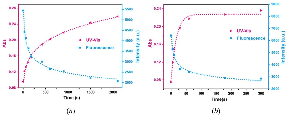
**Figure S21.** Time dependence in peak intensities of UV-Vis diffuse-reflectance (red) and fluorescence (blue) for (a) **1** and (b) **4** under UV-lamp (313 nm) irradiation at different irradiation times.
