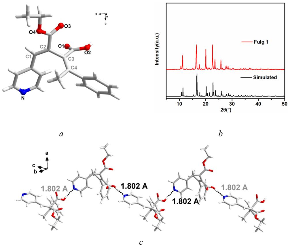
**Figure S18.** (a) Molecular conformation of Fulg1 in Z-form; (b) PXRD pattern for Fulg1; (c) a 1 D infinite zigzag chain fabricated by the hydrogen bonding interactions between neighbouring Fulg1 molecules.
