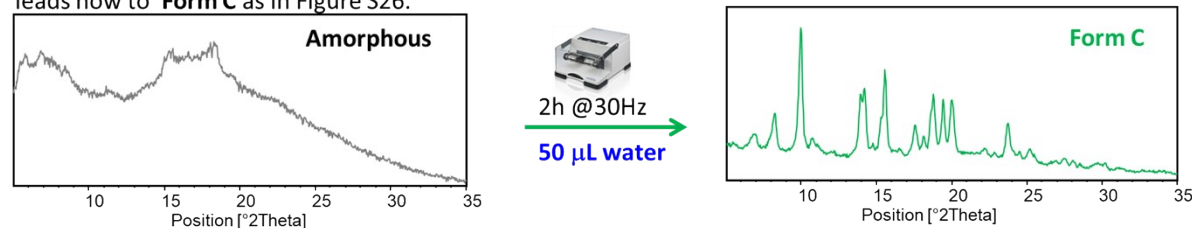
Figure S32. Comparison of the effect of milling the amorphous form under LAG conditions with water to steady-state. a) before the first appearance of Form C leading to the formation of Form B , b) after the first appearance of Form C , obtaining only Form C instead of the disappeared Form B .
