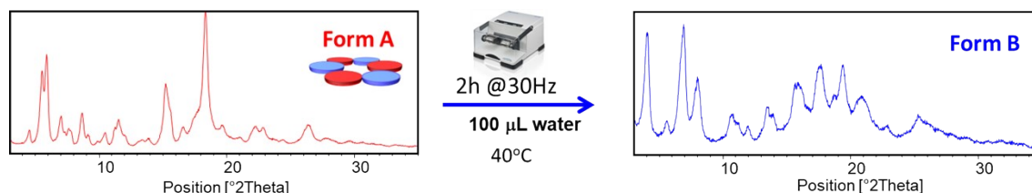
Figure S12. Preparation of Form B by ball mill LAG with water starting from Form A (rosette).
