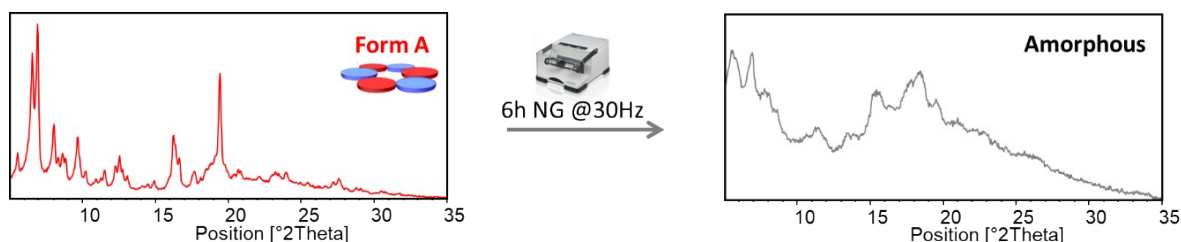
Figure S16. Transformation of Form A to the predominant amorphous form by ball mill neat grinding over extensive milling time to nearly reach a steady-state.
