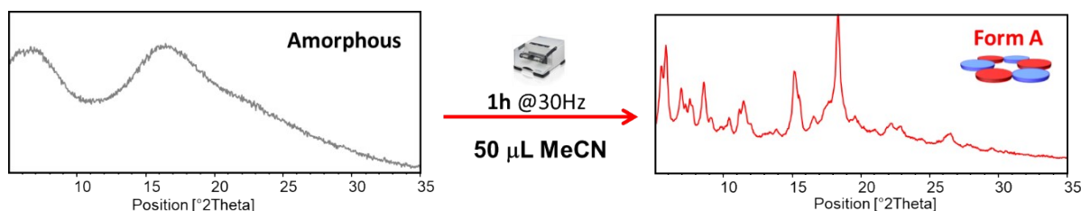
Figure S17. Transformation of amorphous form to Form A by LAG with MeCN.
