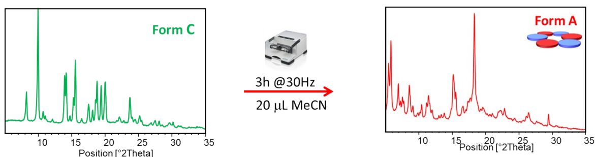
Figure S27. Transformation of Form C to Form A by LAG with MeCN.
