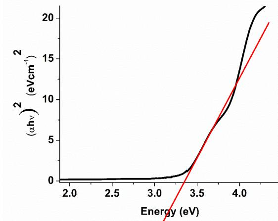
**Figure S2.** Calculation of optical band gap of CP-1 using UV-vis absorption spectrum.
