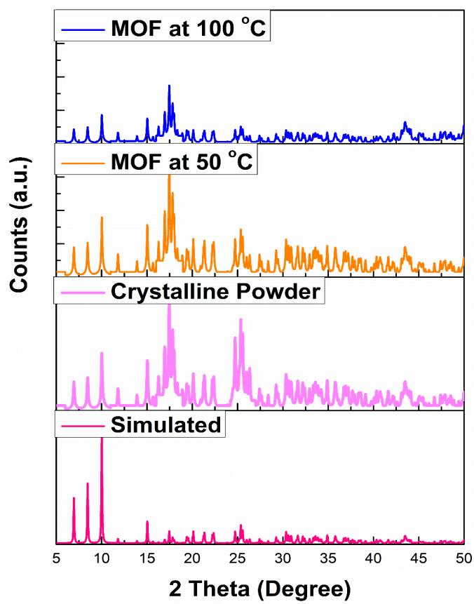
**Figure S11.** PXRD patterns of CP-1 at room temperature (RT), 50 °C, and 100 °C.
