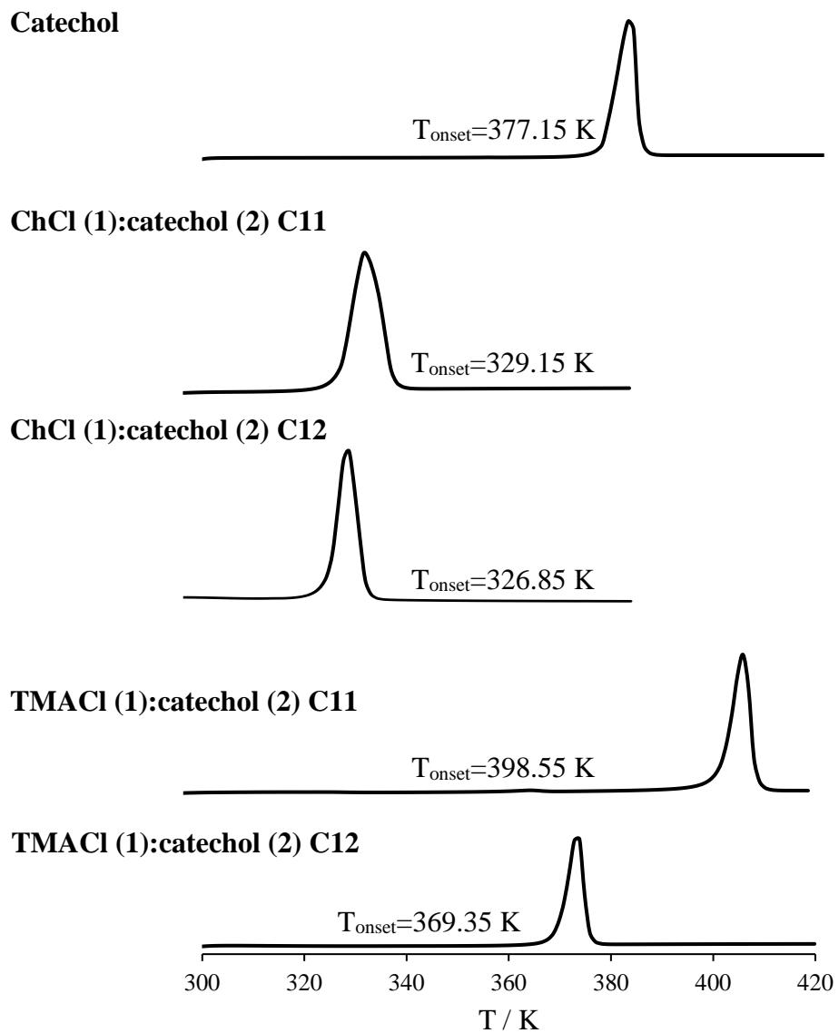
Figure S2. Differential scanning calorimetry curve of cocrystals and pure components.
