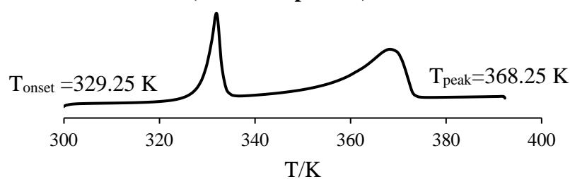
Figure S3. Differential scanning calorimetry curve of solid phase at equilibrium
