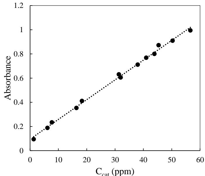
Figure S1. Calibration curve for catechol in acetonitrile, measured by UV spectroscopy.
