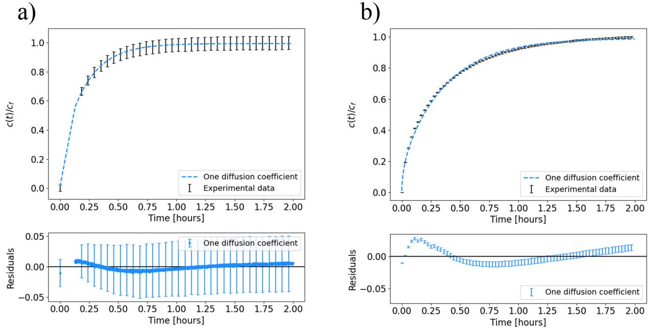
Figure S2: Fitting of the experimental data obtained from conductivity measurements of M25 samples, considering one diffusion coefficient. (a) LiTf electrolyte and (b) LiTFSI electrolyte. Data are plotted in black considering the experimental error bars. The number of measurements were reduced in the graph for better visualization.
