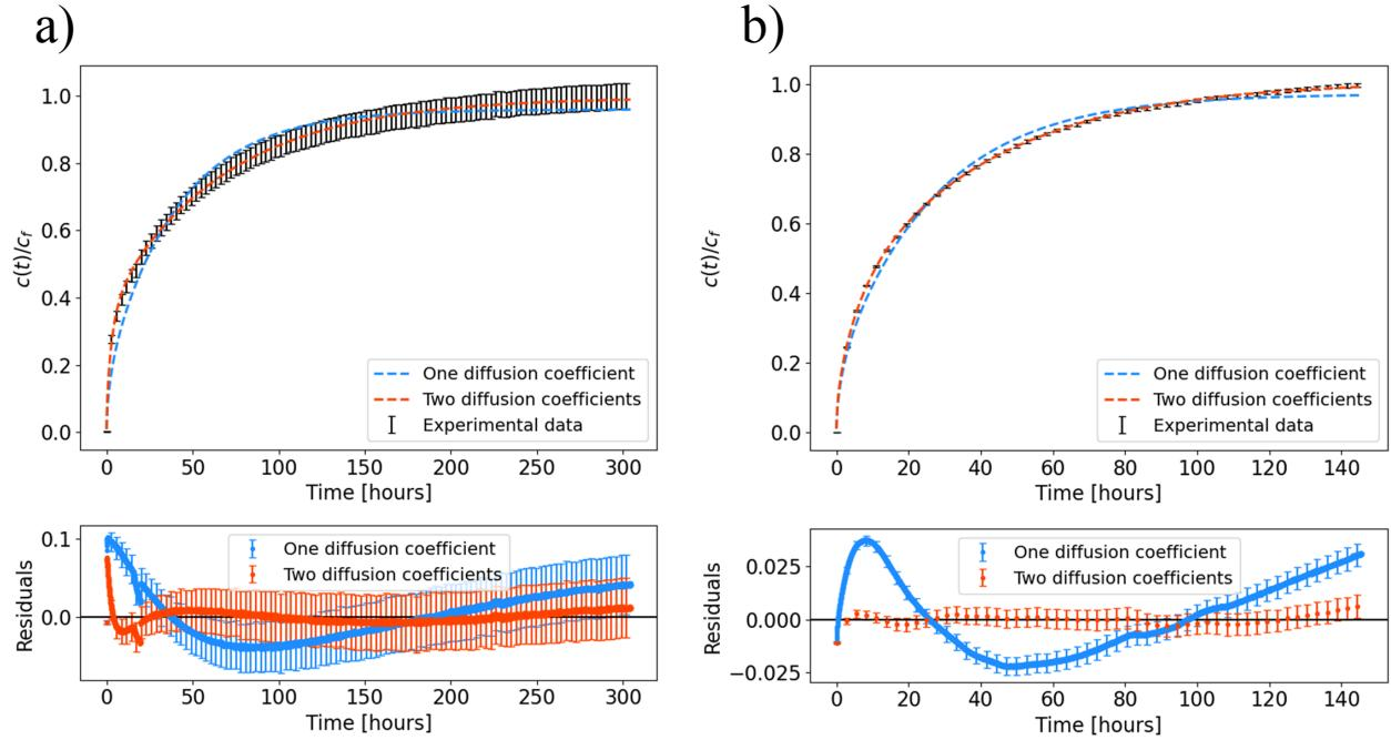
Figure S1: Fitting of the experimental data obtained from conductivity measurements of M4 samples, considering contributions from one (blue) and two (red) diffusion coefficients for (a) LiTf electrolyte and (b) LiTFSI electrolyte. Data are plotted in black considering the experimental error bars. The number of measurements were reduced in the graph for better visualization.
