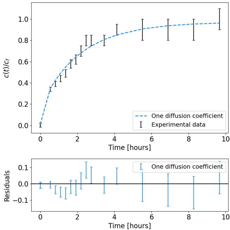
Figure S3: Fitting of the experimental data obtained from conductivity measurements of LiTf electrolyte confined in M10 sample, considering one diffusion coefficient.
