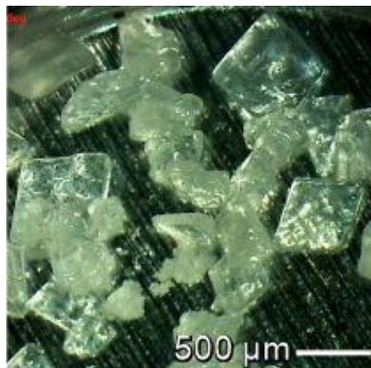
Figure S3. Particle morphology of the CC-DH sample (300–500  $\mu\text{m}$ ).
