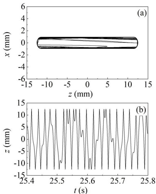
Fig. SI3. (a) Two-dimensional projection of the ball trajectories. Data refer to a ball of 10 mm in diameter and a coefficient of restitution of 0.4. (b) The ball coordinate along the jar main axis,  $z$ , as a function of time,  $t$ . Absolute maxima and minima mark the occurrence of impacts on the hemispherical caps.
