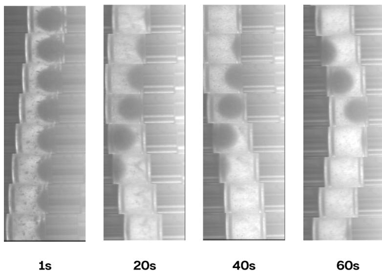
Fig. S15. Time frames of the mechanochemical reactions. The powder flow decreases over time (from left to right).
