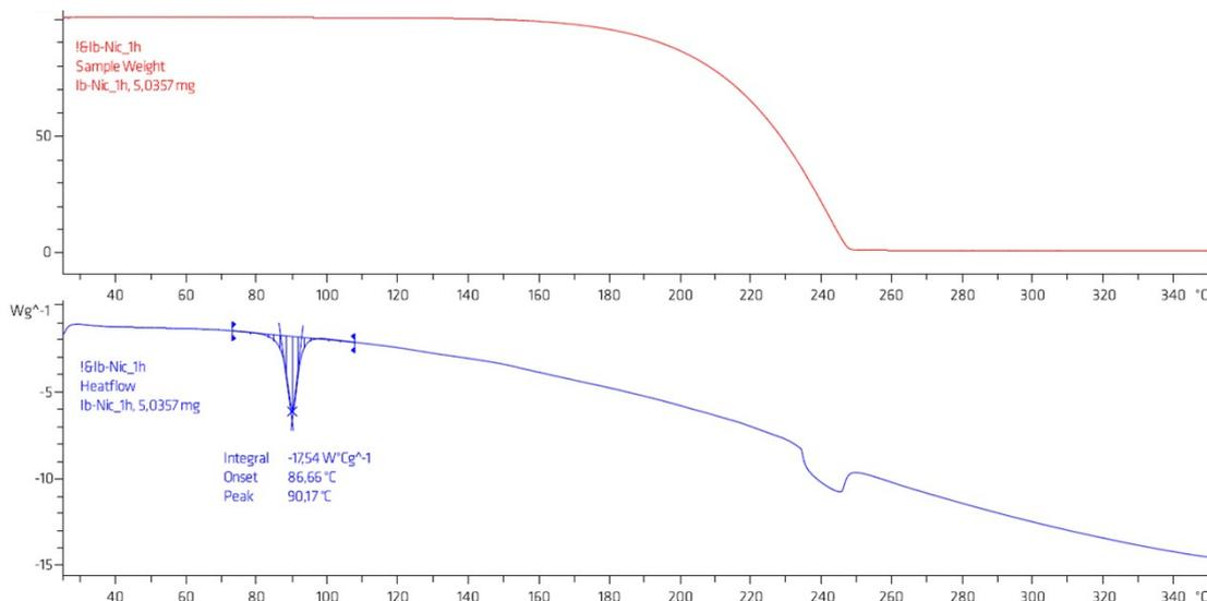
Fig.S14: TGA and DSC profiles for ibuprofen (up), nicotinamide (middle) and the co-crystal ibuprofen-nicotinamide (bottom).
