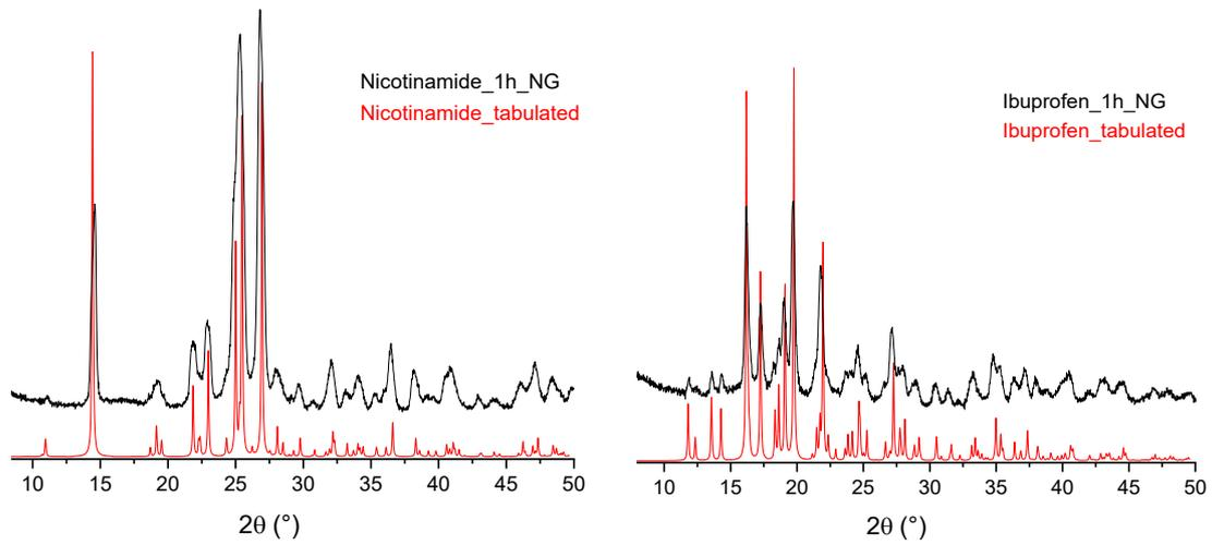
Fig.SI1b. Comparison between the tabulated (black line) and the experimental (red line) pattern for the reagents ibuprofen (up) and nicotinamide (bottom).
