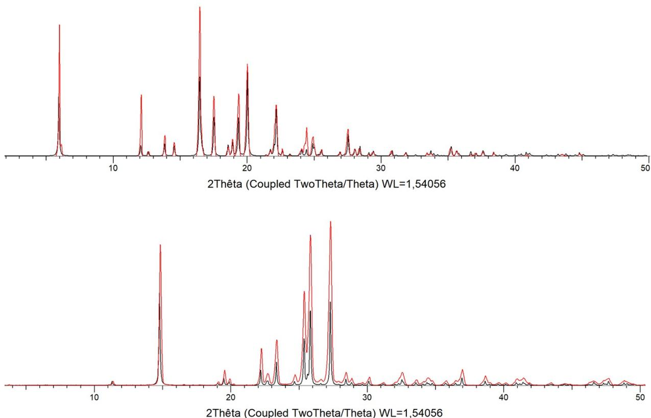
Fig.SI1a. Comparison between the tabulated (black line) and the experimental (red line) pattern for the reagents ibuprofen (up) and nicotinamide (bottom).
