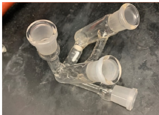
Figure S1. Custom-made CPC electrolysis cell for the quantification of direct ethanol oxidation reaction made from Pyrex glass. All 4 openings have an ID of 12 mm and an OD of 20 mm. All arms have a length of ~80 mm. The working (3 arms) and counter (1 arm) compartments are separated by a glass frit (pore size ~1 micron, diameter 8 mm, thickness 2 mm). The length of the cell is 80 mm. During the CPC measurement, 10 mL of solution is added to the working compartment, while sufficient electrolyte is added to the counter compartment to maintain the same solution height (~ 7 mL) to avoid liquid pressure across the frit. The glassy carbon disk working electrode is inserted to the cell through the middle opening, while the reference is placed in the left-most opening. The distance between the working and reference electrodes is purposely held at 10 mm. The CPC experiments are conducted without IR compensation, and all reactions are carried out in an air-conditioned room held at 20° C.
