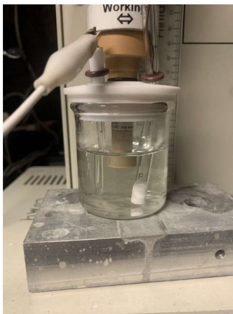
Figure S2. RRDE setup with CHI760E potentiostat and RRDE-3A from ALS Japan. The volume of electrolyte solution is always 50 mL. Both the reference and the counter electrodes are separated from the bulk solution by fine glass frits.
