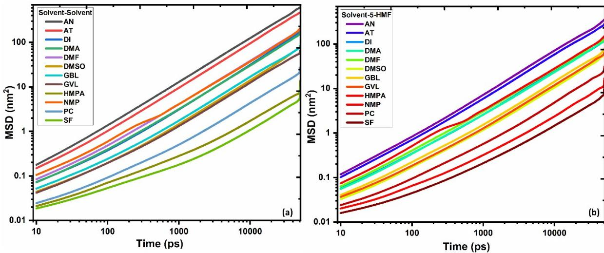
**Figure S3.** Mean square displacement on a log-log scale of 5-HMF with (a) different solvent systems, and (b) 5-HMF.
