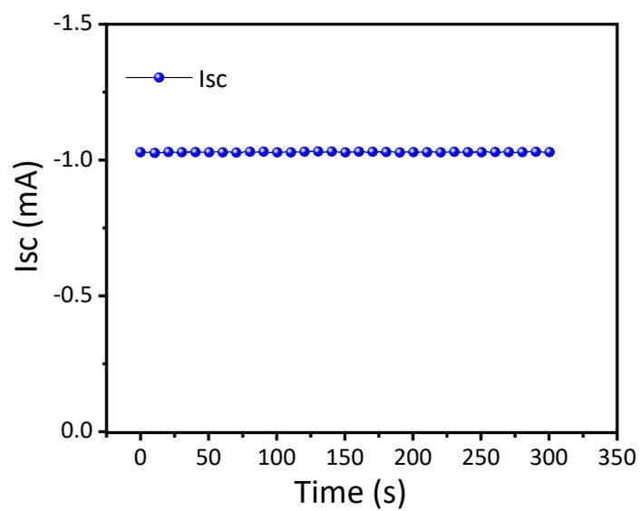
**Figure S4.** Steady-state current output of the champion device.
