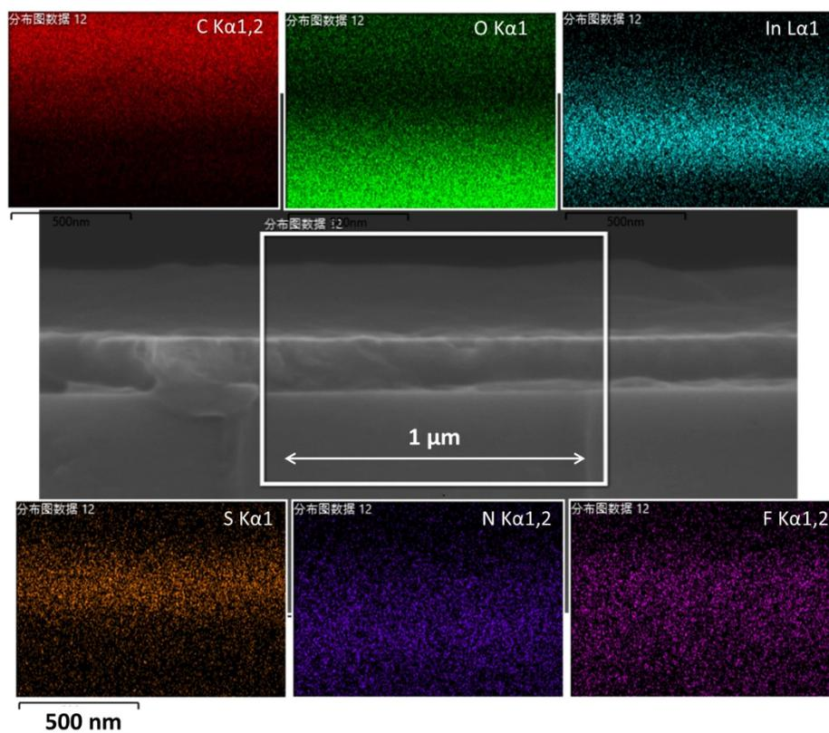
**Figure S6.** Elemental mapping of cross-section of the active layer without DIO.
