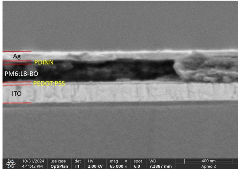
**Figure S8.** Cross-section SEM figure of the fabricated device. Confirming the device architecture of ITO/PEDOT:PSS/PM6:L8-BO/PDINN/Ag.
