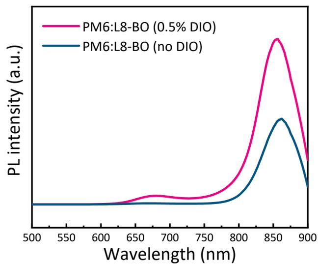
**Figure S7.** PL of the active layer with and without DIO. Excitation: 460 nm.
