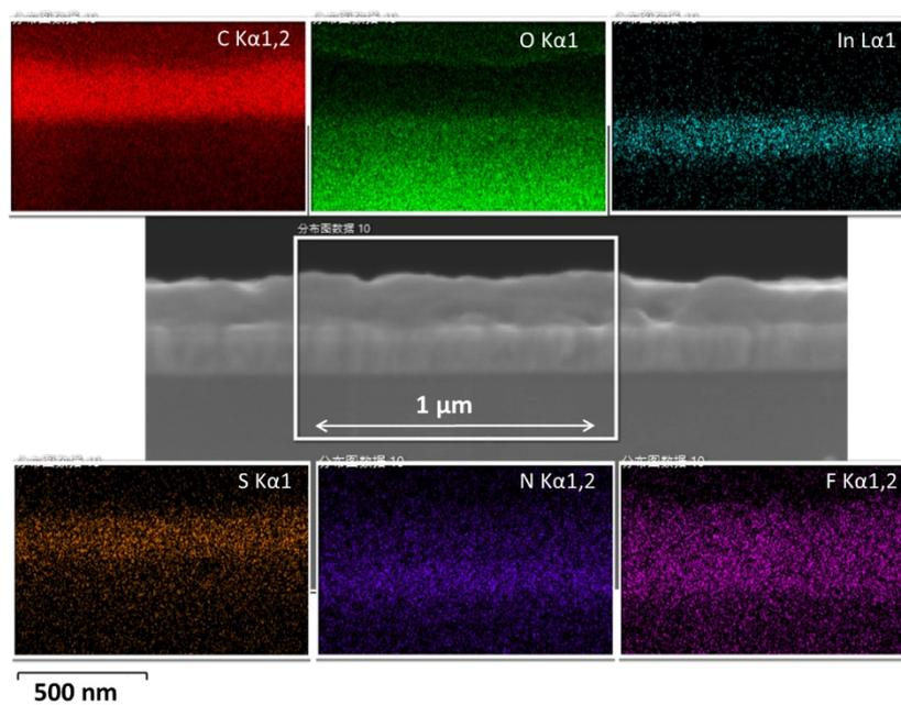
**Figure S5.** Elemental mapping of cross-section of the active layer with DIO.
