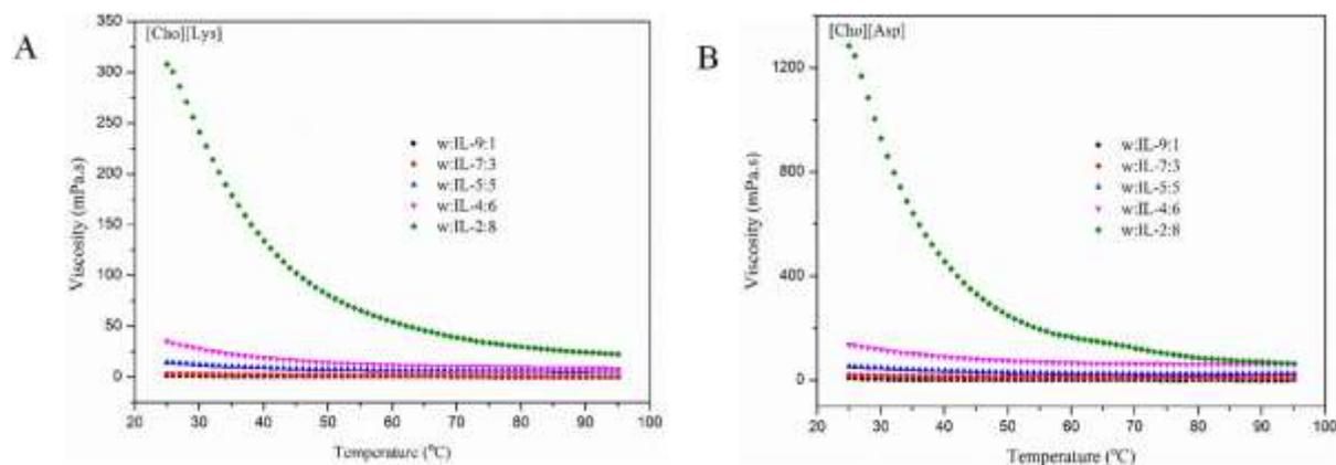
Fig.S5 The effect of temperature on the viscosities of [Cho][Lys]-water (A) and [Cho][Asp]-water (B) solvents.
