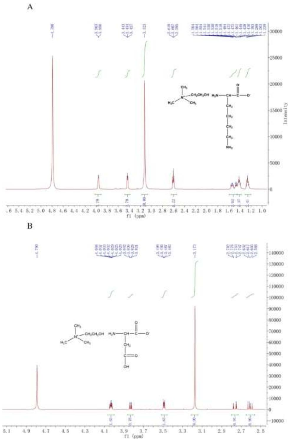
Fig.S3  $^1\text{H}$  NMR spectra of [Cho][Lys] (A) and [Cho][Asp] ILs (B).
