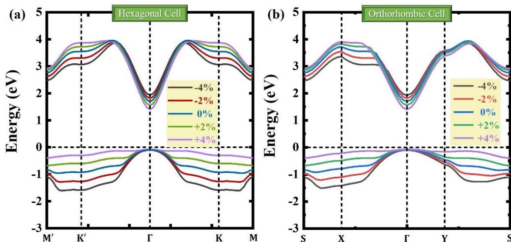
Figure S2. Effect of strain on lowest conduction band (LCB) and highest valence band (HVB) in (a) hexagonal unit cell and (b) orthorhombic unit cell
