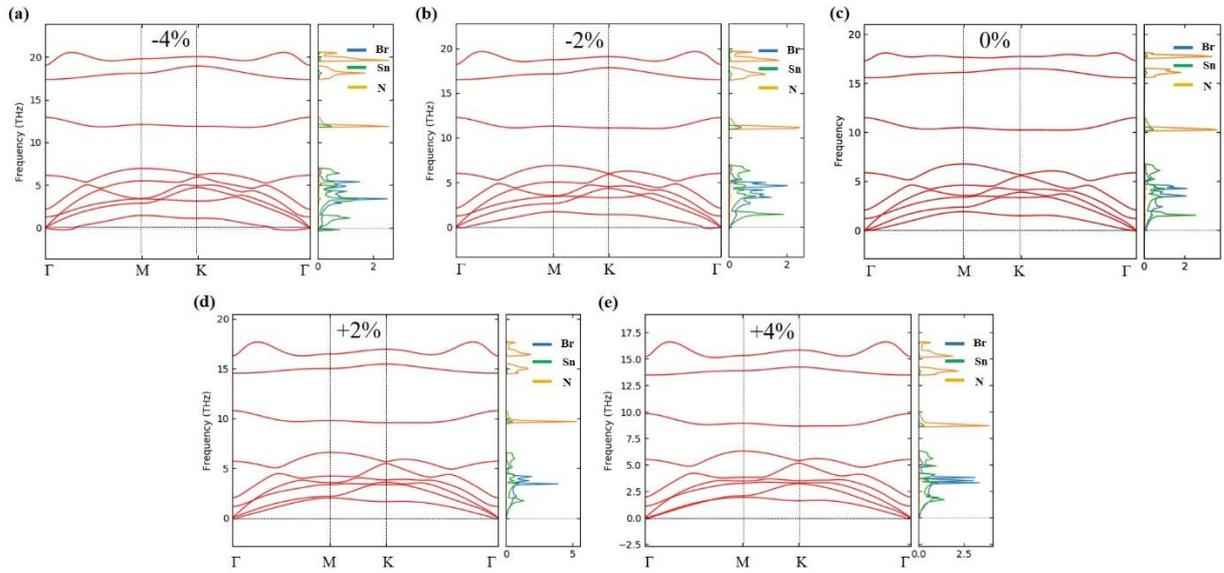
Figure S1. Phonon dispersion of the strained SnNBr monolayer under the (a) compressive biaxial strain 4%, (b) compressive biaxial strain 2%, (c) unstrained condition or 0%, (d) tensile biaxial strain 2%, and (e) tensile biaxial strain 4%.
