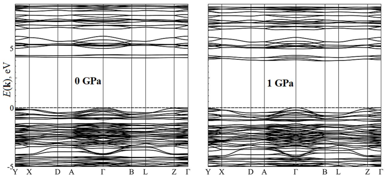
Fig. S2. Band structure of TBPA crystal at pressures of 0 and 1 GPa.
