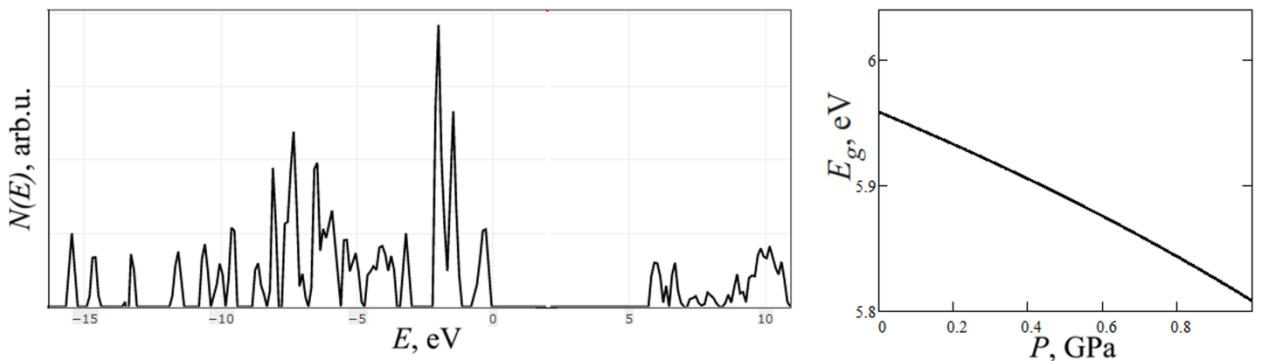
Fig. S5. Density of states  $N(E)$  and the pressure dependence of the band gap for EMN crystal.
